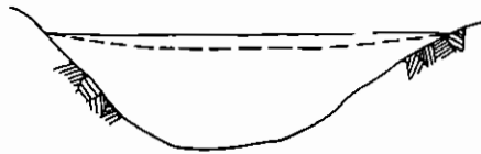
(a) Near-uniform settlement of a dam.
