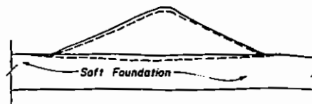
(h) Settlement of foundation.
