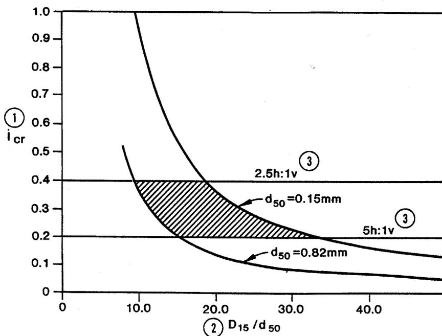
Figure 6 Critical gradient with steady flow parallel to the interface (ICOLD 1994 based on Bakker 1987)
