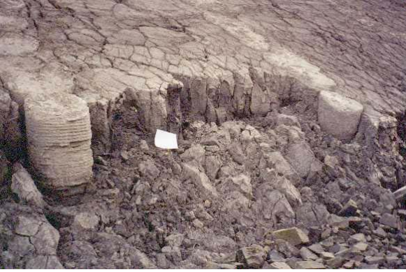
Fig.15 Soil Stabilization Using Lime-Cement Piles (left); Three Dimensional Finite Element Modelling of the interaction between the reinforcing lime-cement ribs and surrounding soil (right).
