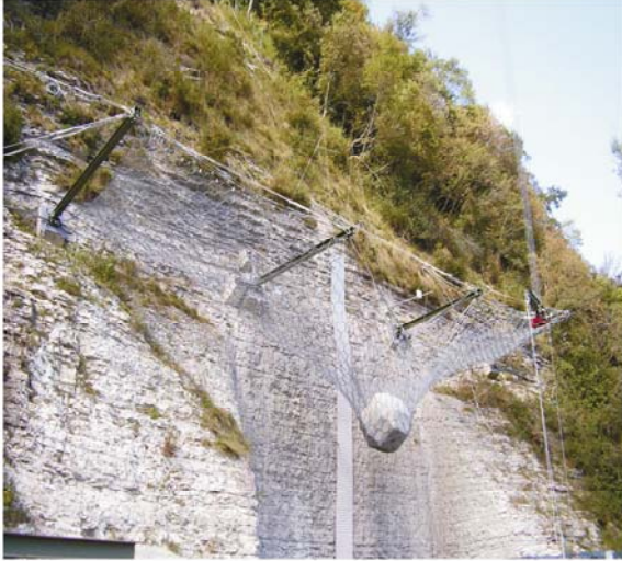
Fig.16 Full Scale Modeling of the Behavior of the Rockfall Protection Fences: Rock blocks of different sizes are dropped vertically onto the protection net to assess its deformation and breaking time.
