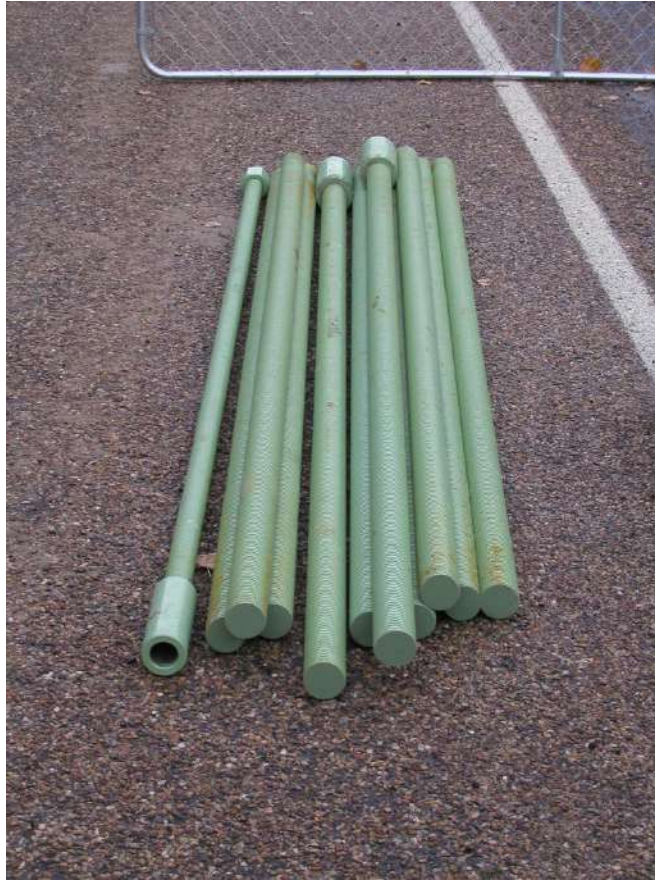
Figure 14-5.—Epoxy coated rock bolts (Reclamation).
