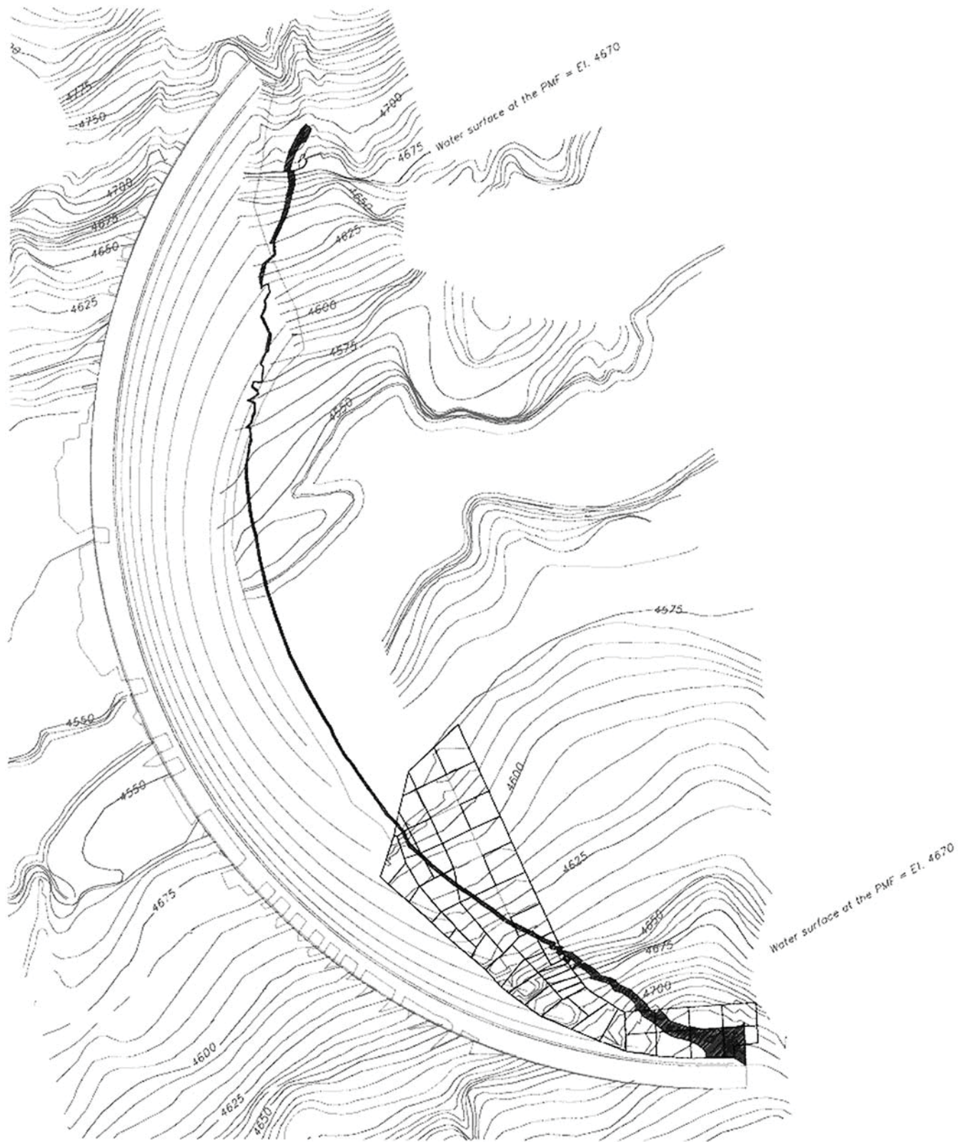
Figure Gibson-5 - Footprint of the trajectory with no spread of the jet for the PMF overtopping (Reclamation, 2006).
