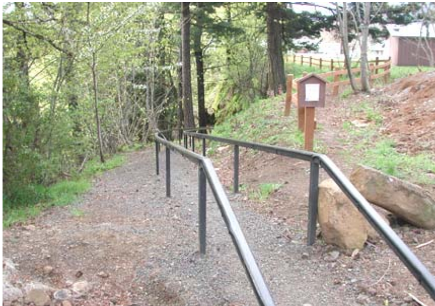
Photo 10I: Parallel metal bars serve as a boatslide while designating the portage trail
