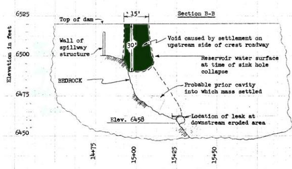
Figure 19: Section B-B of the sinkhole looking upstream.
