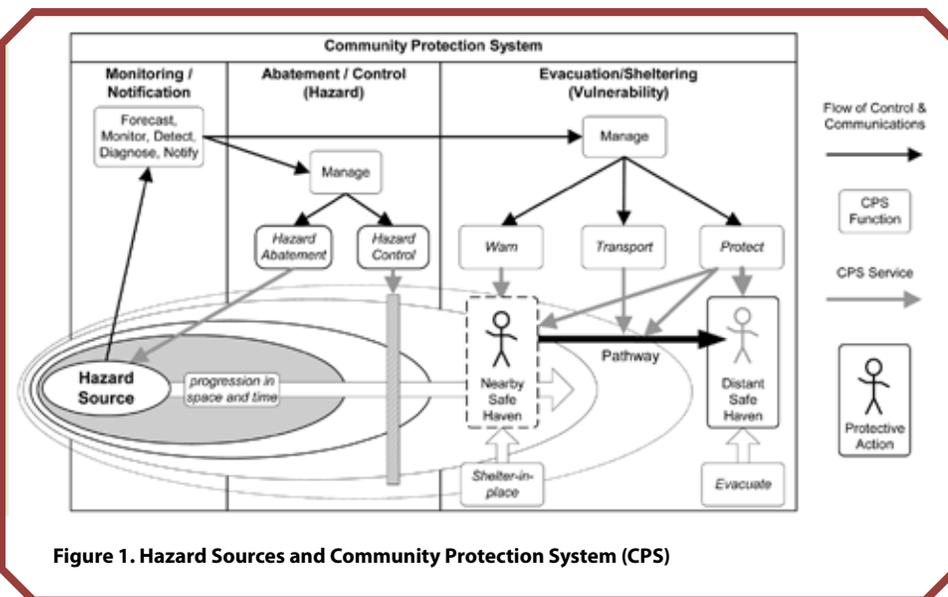
Figure 1. Hazard Sources and Community Protection System (CPS)
