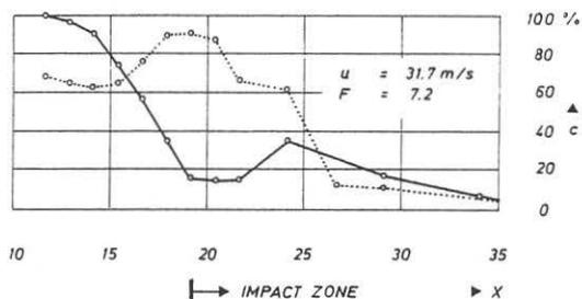
Fig.17. Air concentration distribution along channel bottom.
