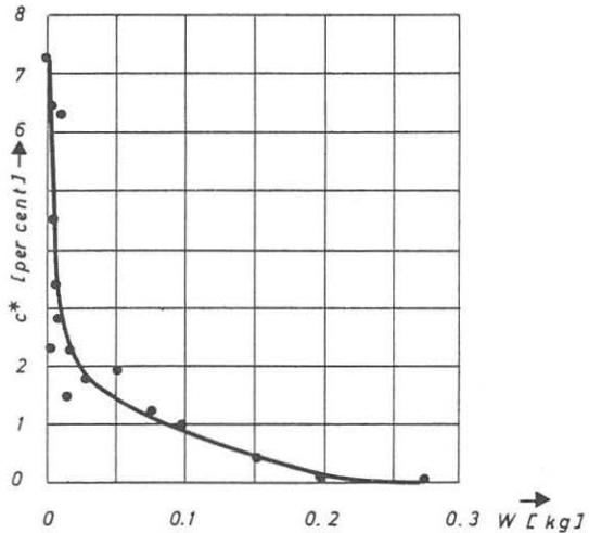
Fig.12. Air content versus cavitation weight loss of concrete specimens (according to Peterka A.J., 1953).
