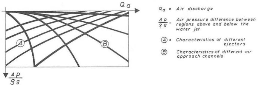
Fig. 7. Characteristics of a water jet aspirator (principle)
