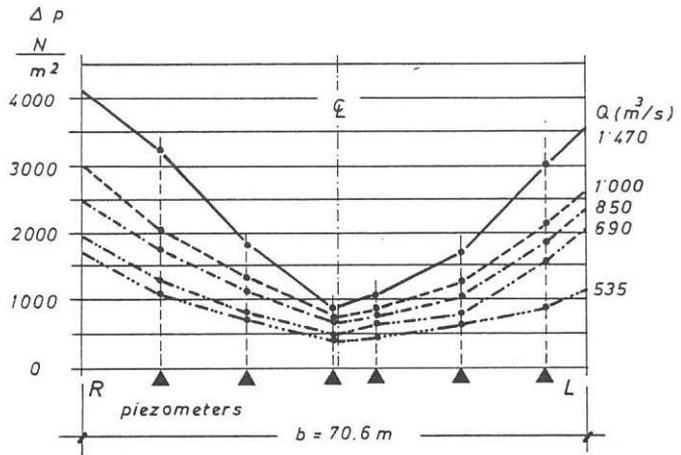
Fig. 11. Pressure distribution below the water jet. Symmetrical air flow conditions.
