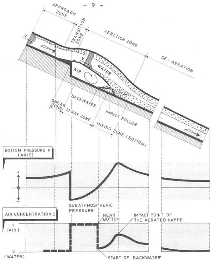
Fig. 2. Air entraining mechanism by an air slot. (Principle of air slot operation).
