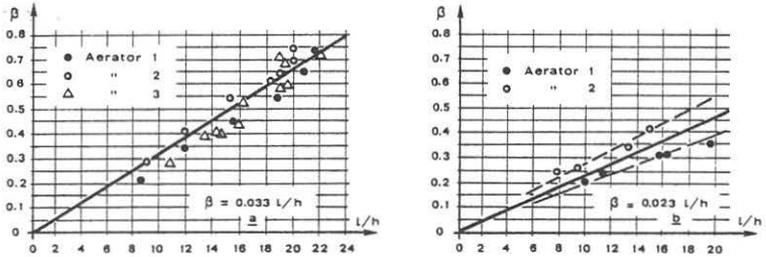
Fig. 6.  $\beta = f(l/h)$  as estimated from prototype results.
