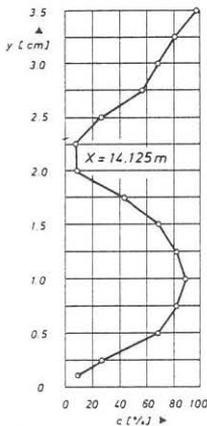
Fig. 14. Example of air concentration profile for  $\text{tg } \alpha = 1:4$ ,  $q_w = 40 \text{ m}^3/\text{ms}$ ,  $t_r = 0.50 \text{ m}$ ,  $t_s = 0.75 \text{ m}$ . (according to Vischer, Volkart, Siegenthaler, 1981).
