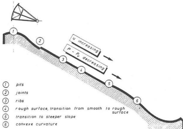
Fig. 1. Possibilities for cavitation erosion on an open chute spillway.
