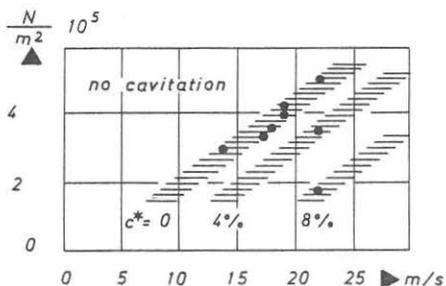
Fig.13. Relation between allowable velocities of a cavitation flow, the concrete strength and the air content  $C^*$  (according to Galperin, R.S. et al 1971).  $C^*=100 \cdot$ air volume/water volume.
