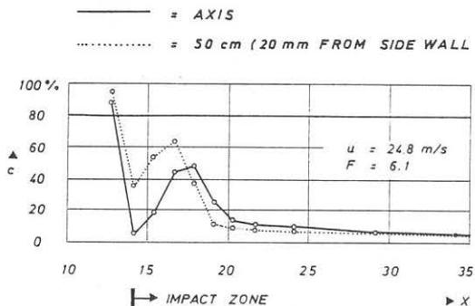
Fig. 16. Air concentration distribution along channel bottom. (10 cm above the bottom).
