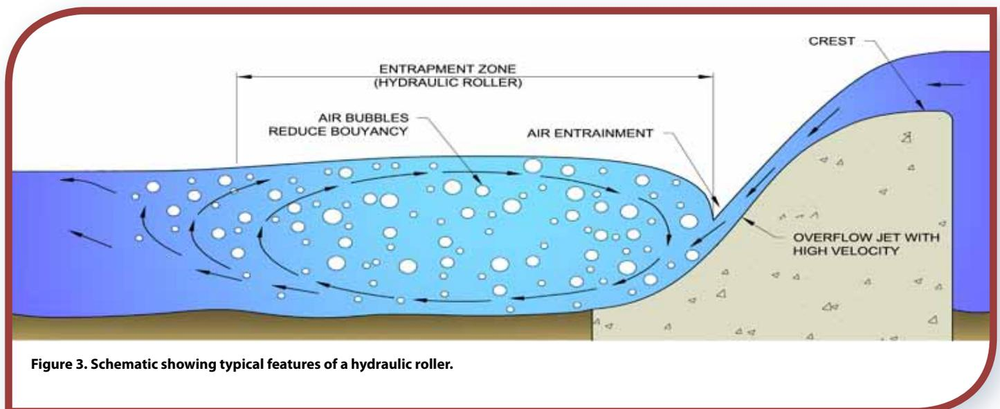
Figure 3. Schematic showing typical features of a hydraulic roller.
