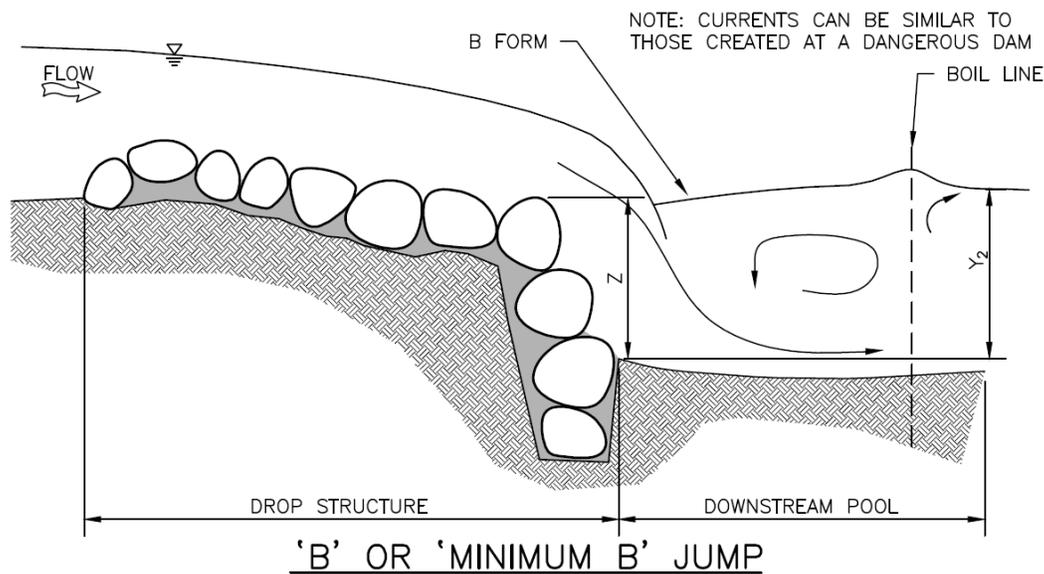
THIS FORM CAN BE BENIGN OR CREATE A PLUNGING OR DIVING JET (AS ILLUSTRATED) THAT CAN BE OVERLY-RETENTIVE AND HAZARDOUS. THIS IS OFTEN CAUSED BY A LOWER THAN PREDICTED TAIL WATER ELEVATION ( $Y_2$ ) OR DOWNSTREAM DEGRADATION OF THE CHANNEL OR RIVER BED.
