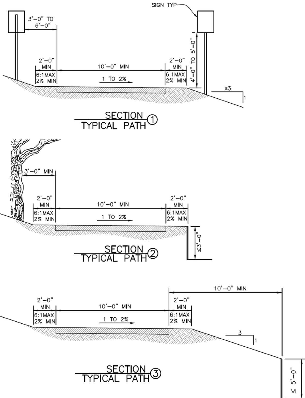
Figure 10-3. Typical path sections 1, 2, and 3.
