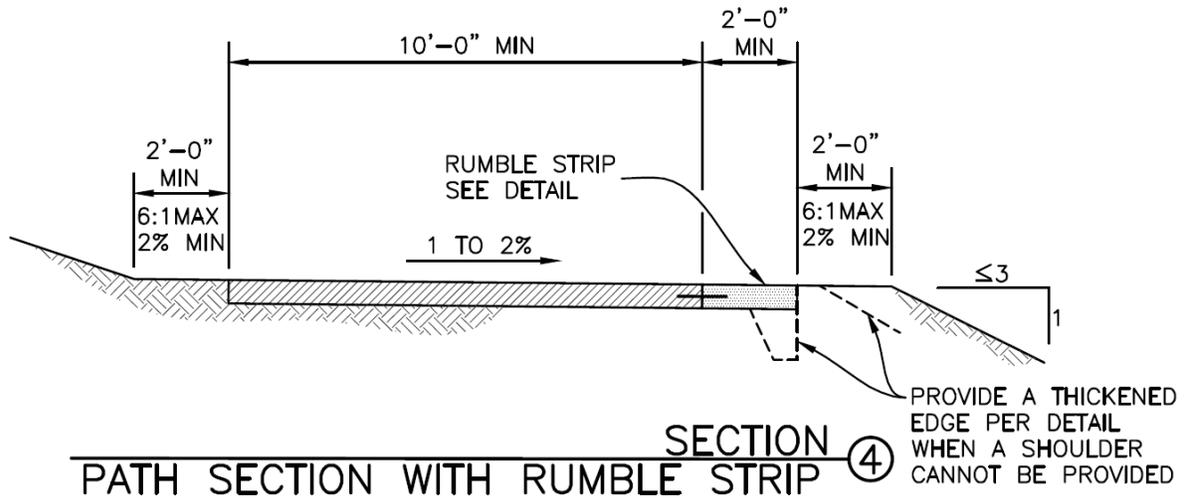
Figure 10-4. Path section with rumble strip
