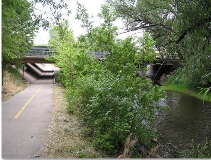
**Photograph 10-9.** Striping used sparingly can be effective in alerting the user of a safety concern. In this photo, it is used where the path approaches a crossing.
