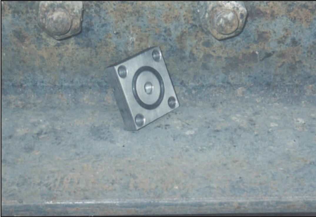
Photograph No. 6.—Grease block fitting with “O” ring installed.
