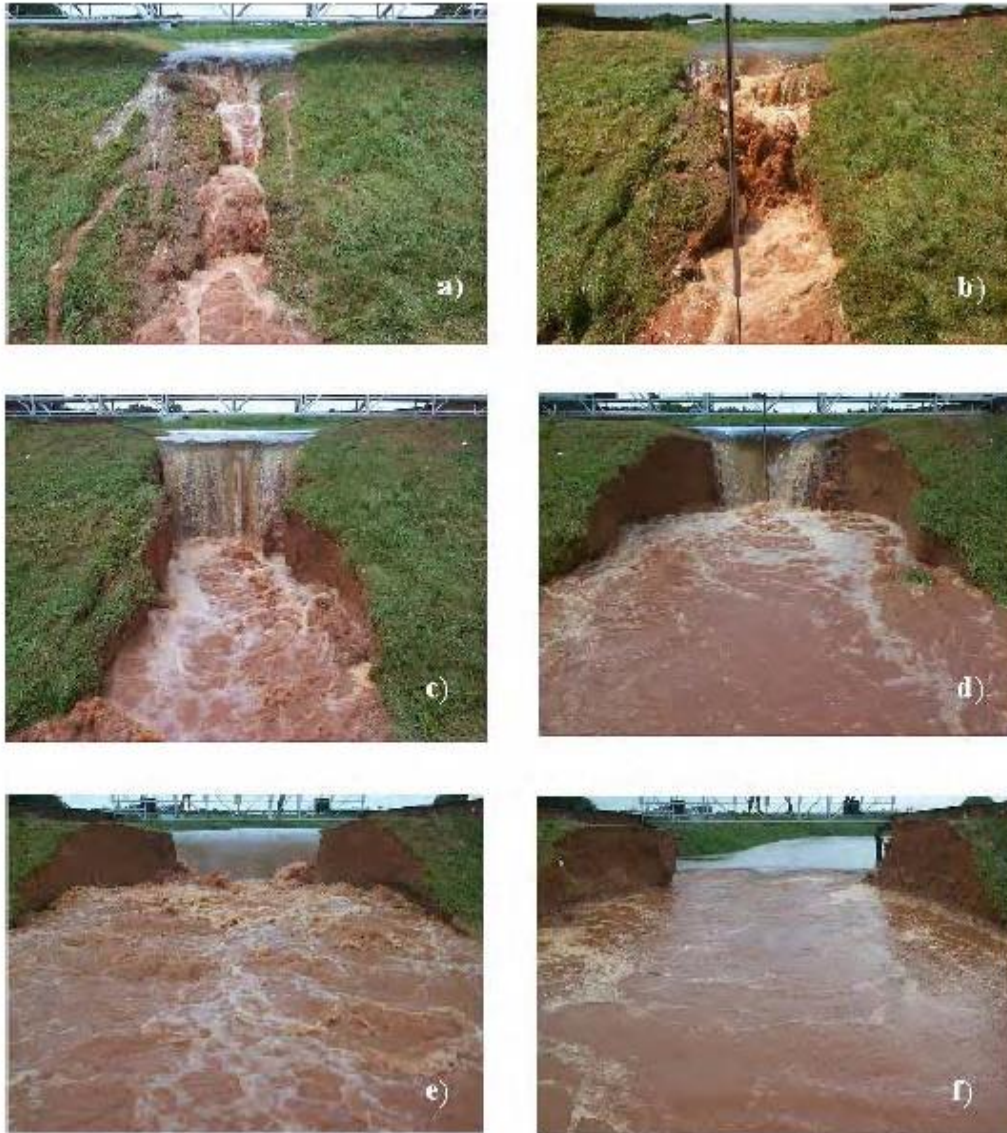
Figure D-1-9 – Generalized description of observed erosion processes during ARS overtopping tests: a) rills and cascade of small overfalls during Stage I, b) consolidation of small overfalls during Stage I, c) headcut at downstream crest, transition from Stage I to Stage II, d) headcut at upstream crest, and f) transition from Stage III to Stage IV at breach formation (Hanson et al 2003).
