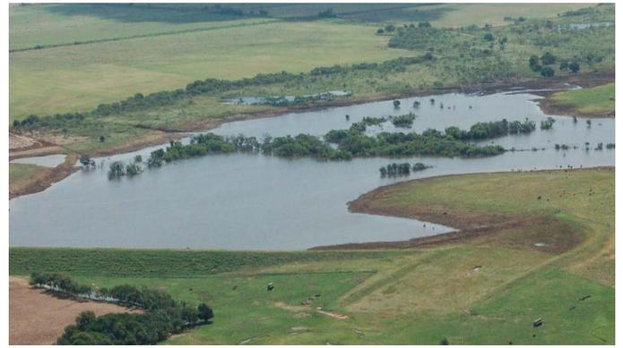
Figure 5: Auxiliary spillways are typically vegetated channels that safely convey runoff from large storms around the dam to avoid overtopping of the embankment
