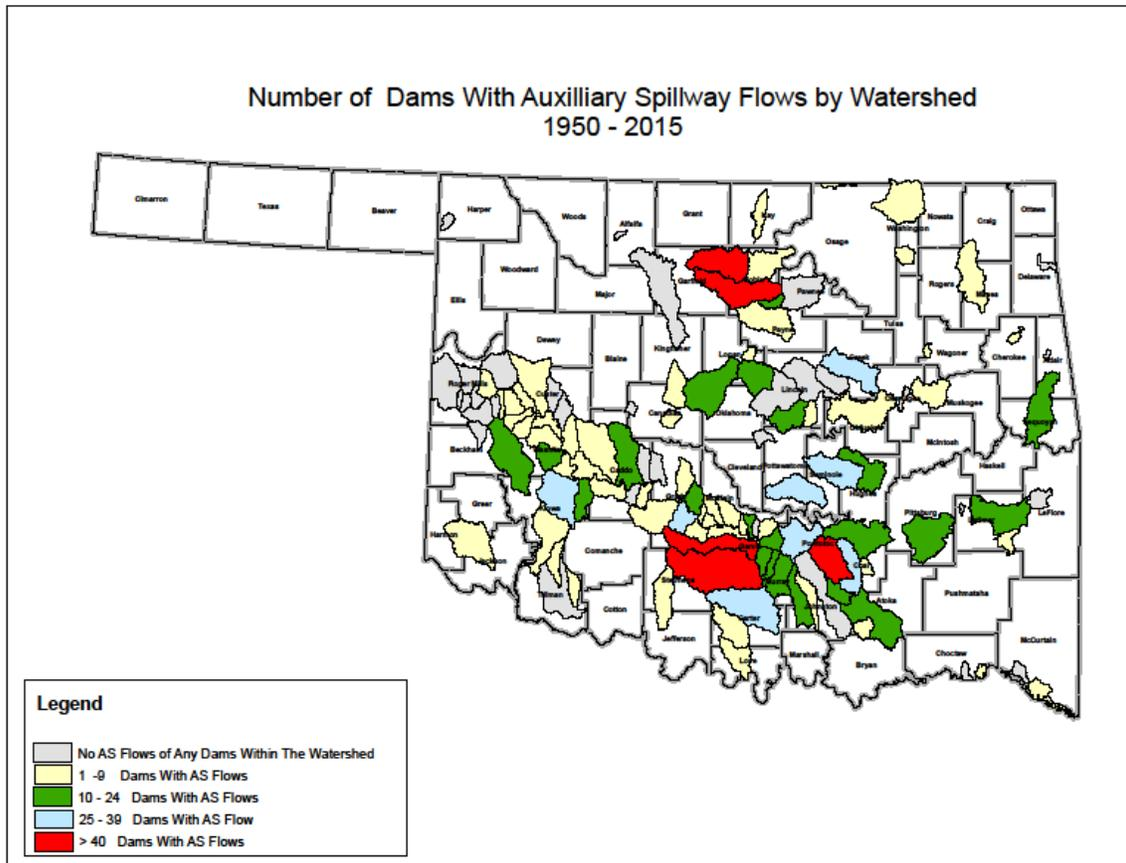
Figure 11: Watershed projects with dams showing number of auxiliary spillway flows
