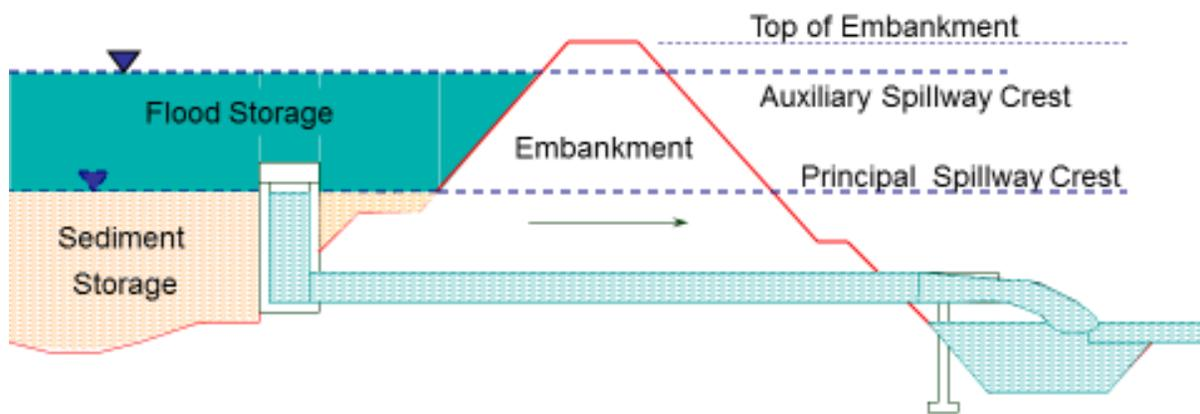
Figure 3: Section of Typical Watershed Dam
