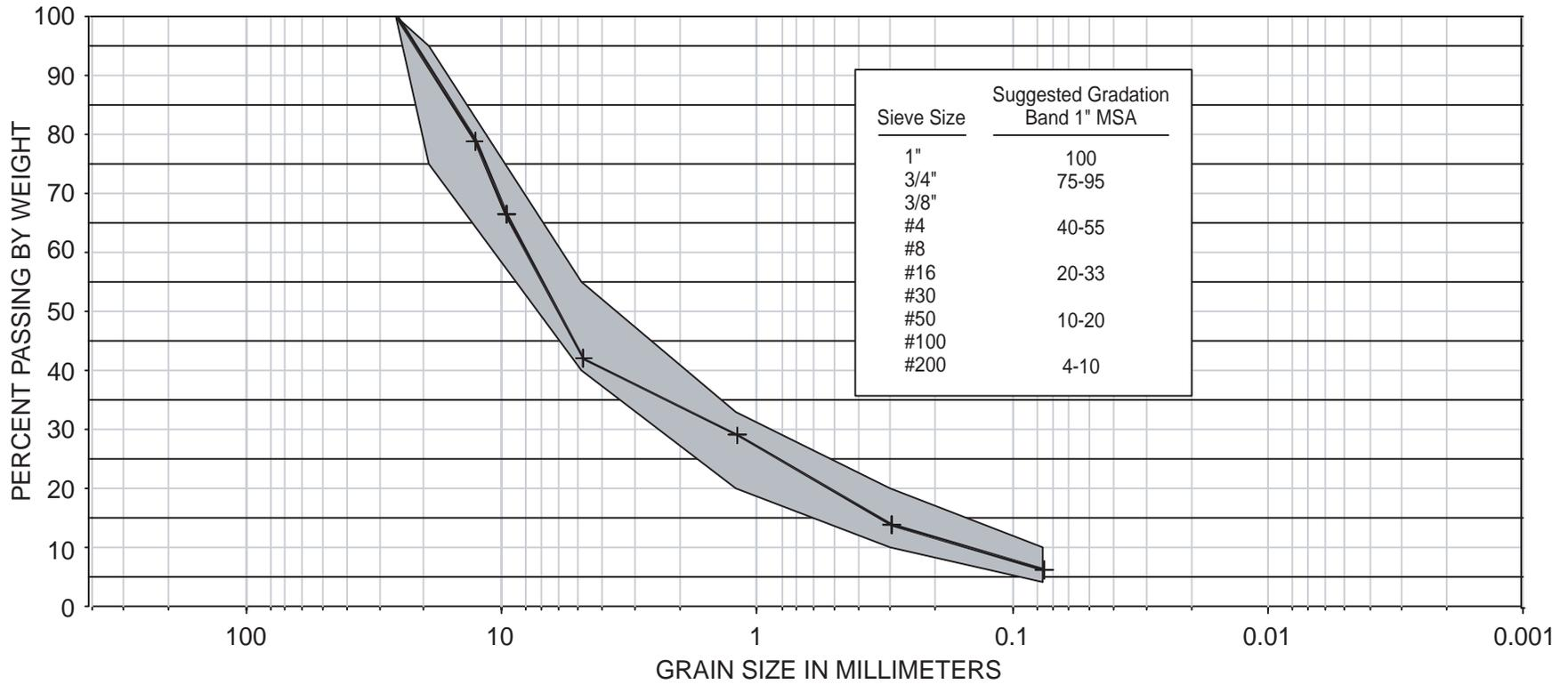
Figure A.7. RCC aggregate gradation example
