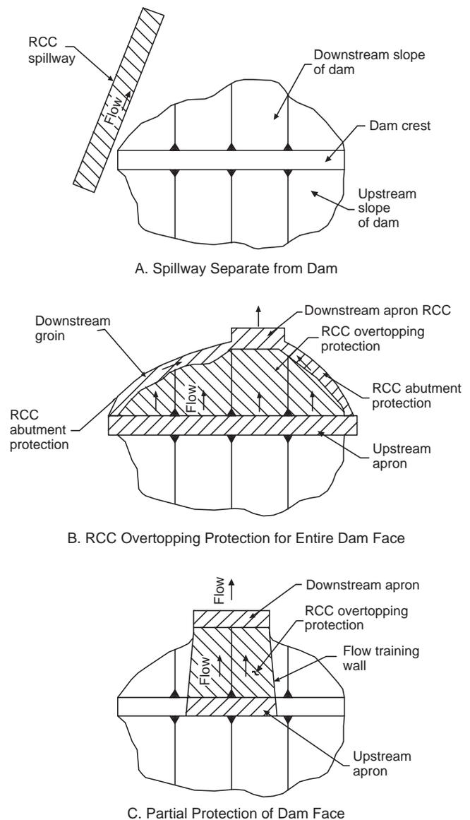
Figure 6.1. Alternative spillway locations.
