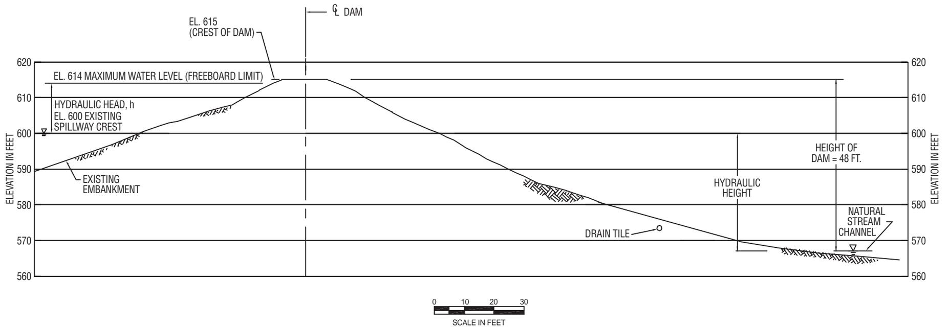
Figure A.1. Typical Dam – Existing cross section
