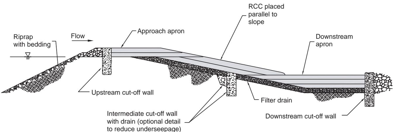
Figure 6.4. Overtopping protection with RCC placed parallel to chute (plating).
