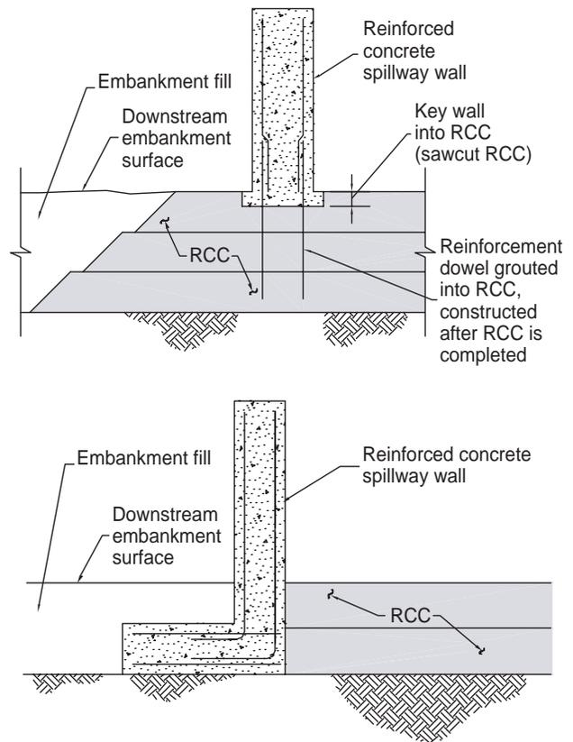
Figure 6.41. Reinforced concrete training wall (section looking downstream).
