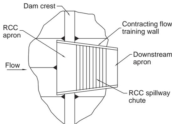
B. Plan of Contracting Spillway Walls
