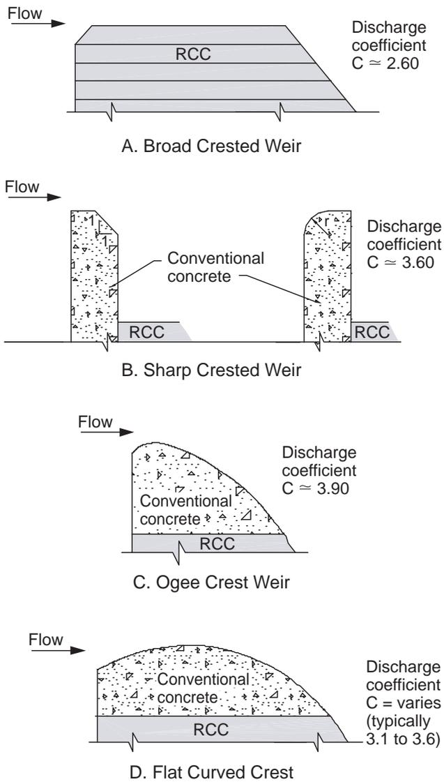
Figure 6.16. Alternative weir crest shapes.
