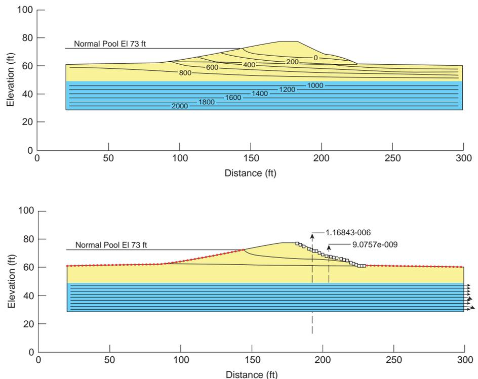
Figure 5.5. Example of results from SEEP/W finite element seepage analysis.
