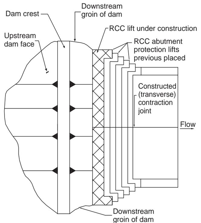
Figure 6.31. Plan of RCC overtopping and abutment protection partially constructed.
