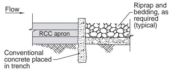
A. Conventional Concrete Cut-off Wall
