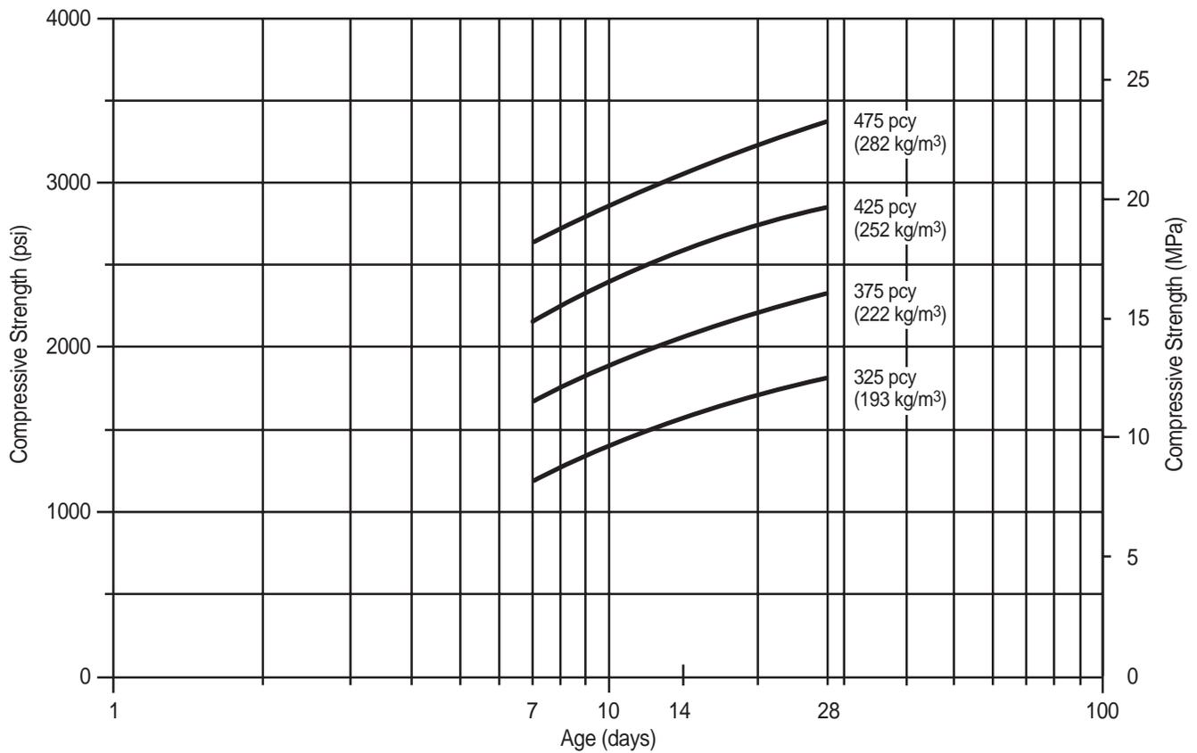
**Figure A.10. RCC compressive strength versus age for various cement contents – conventional concrete method**
