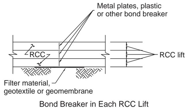
Figure 6.30. Typical section at contraction joint.
