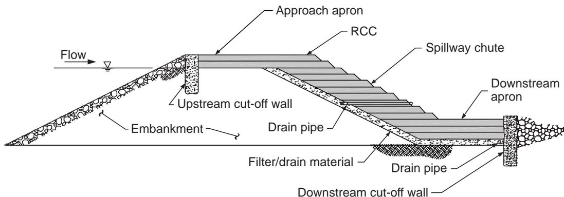
Figure 6.2. Typical section: RCC overtopping protection.
