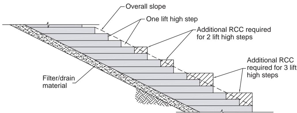
Figure 6.9. Step height comparison of RCC volume.
