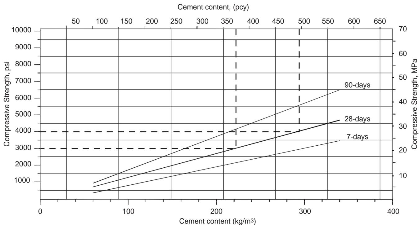
**Figure A.9. Compressive strength versus cement content for various ages**
