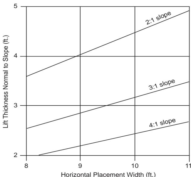
**Figure 6.13. Thickness of RCC on the slope versus the width of the lift.**
