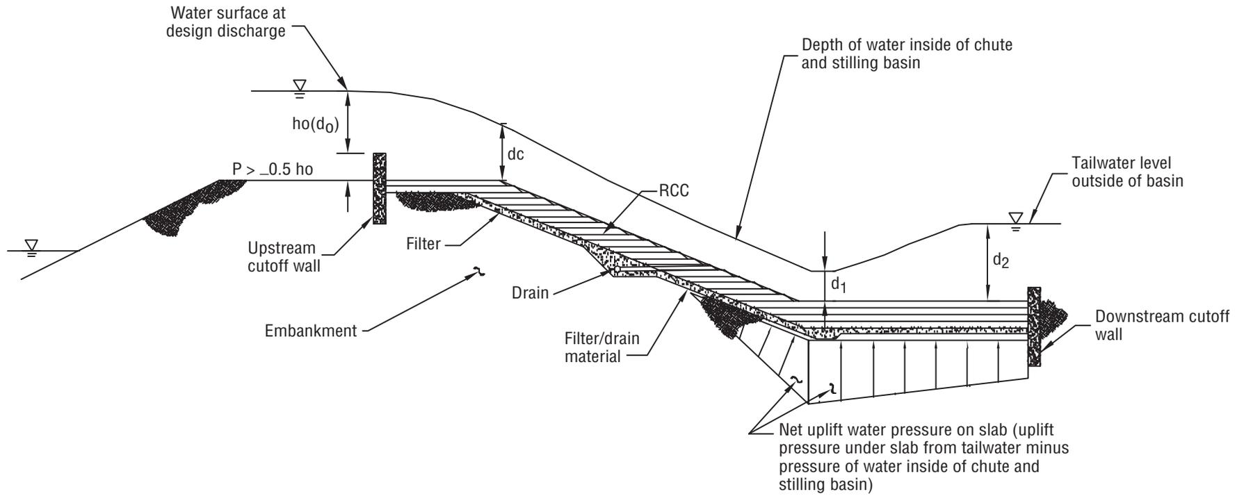
Figure A.6. Hydraulic design parameters
