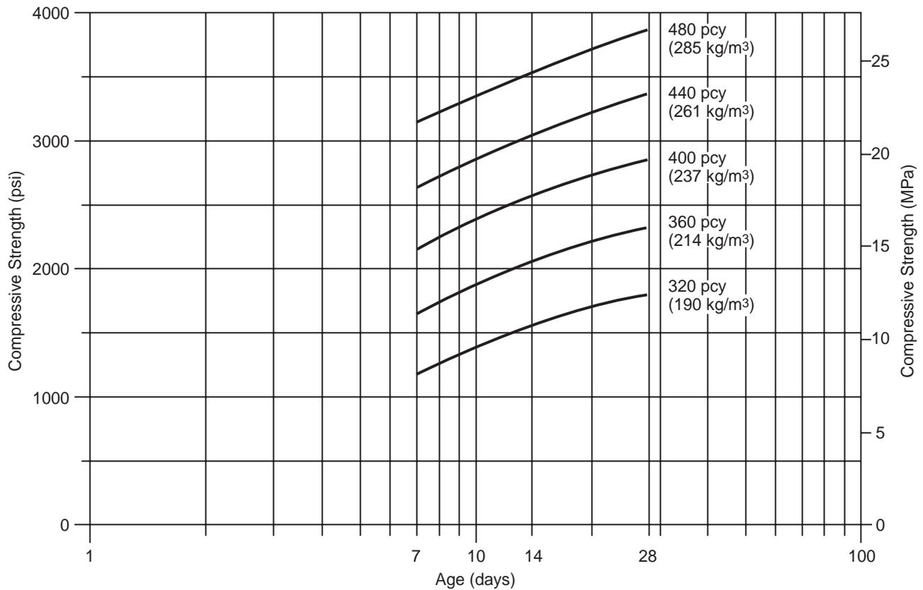
**Figure A.8. RCC compressive strength versus age for various cement contents – soil compaction method**
