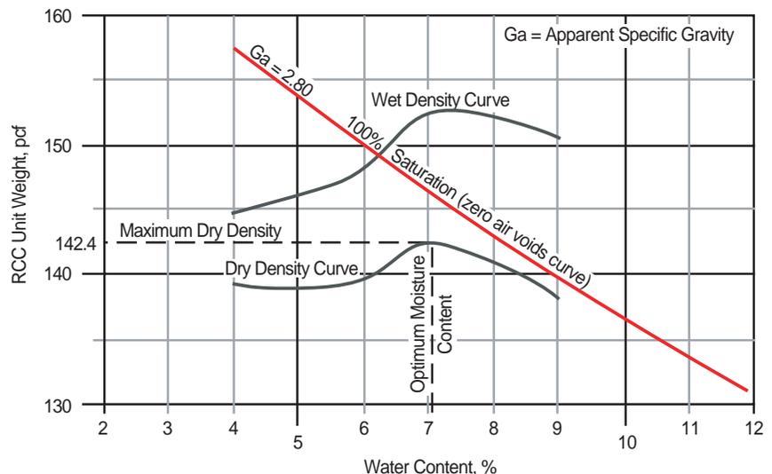
Figure 7.1. Typical RCC moisture-density relationship (ASTM D 1557).
