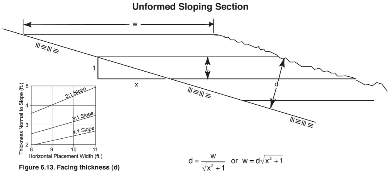
Figure 6.13. Facing thickness (d) of RCC versus width (w) for a 1-ft thick (L) unformed sloping RCC step.
