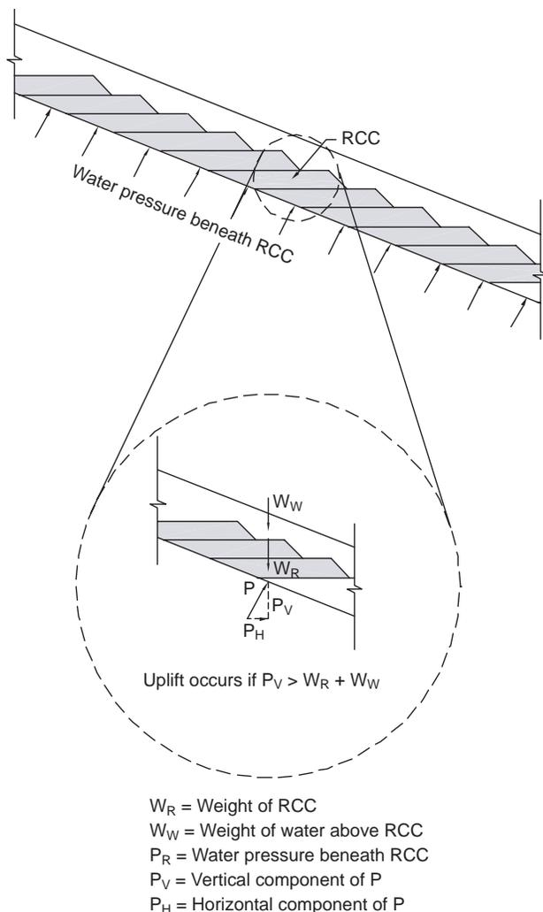
Fig. 5.6. Physics of uplift for RCC overtopping protection.
