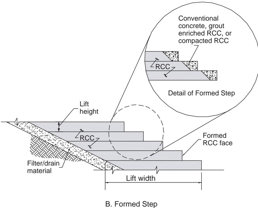
Figure 6.3. Downstream slope geometry of RCC overtopping section.
