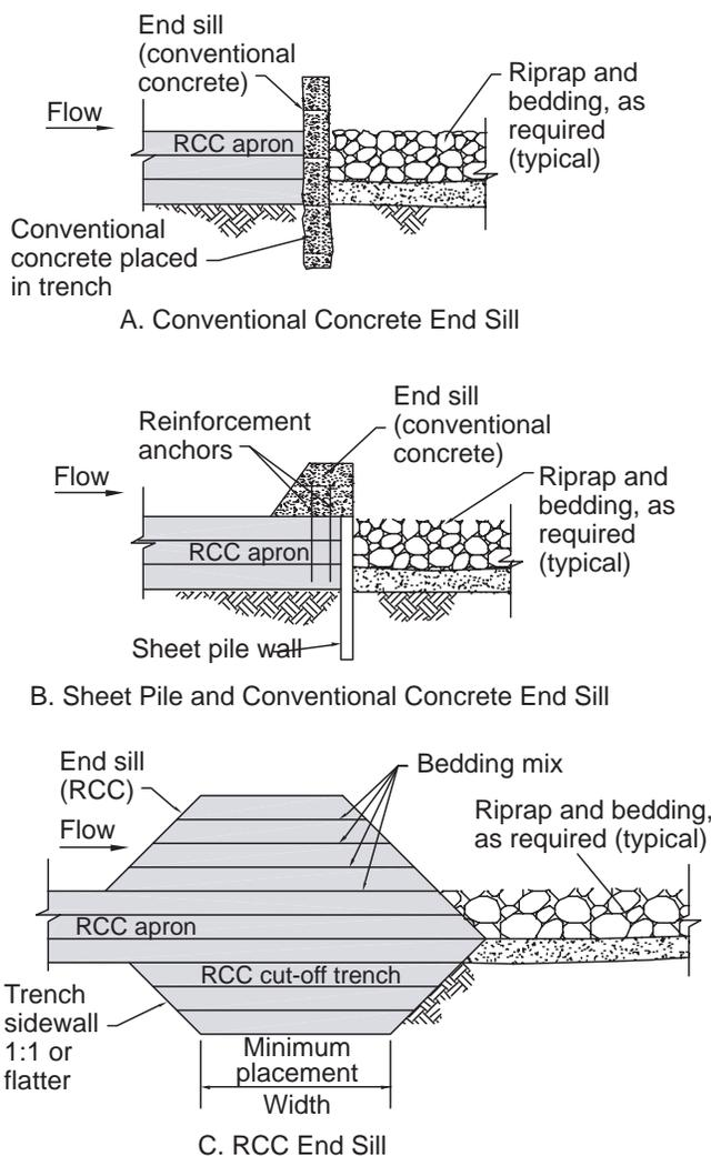
Figure 6.28. Alternative end sill details.
