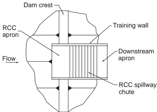
A. Spillway Walls Parallel to Flow
