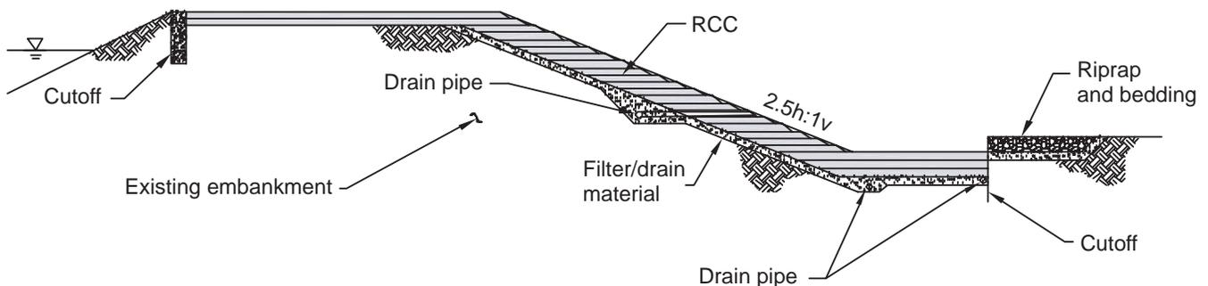
**Figure 5.3. Typical RCC overtopping section with underdrain (not to scale).**
