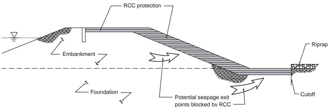
Figure 5.1. Seepage exit points blocked by RCC overtopping protection.
