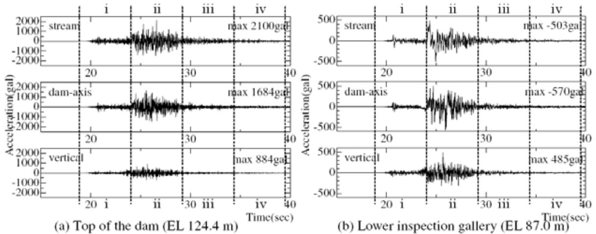
Figure 8. Acceleration time histories measured at Kasho Dam (from Yamaguchi et al., 2002)
