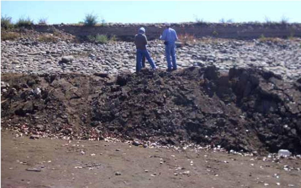
Figure 6. Scarp and bulge (from Bray et al., 2010).
