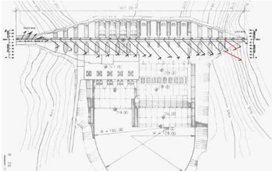
Figure 2. Movement along the dam crest observed in 2009 (from ICOLD 1998).
