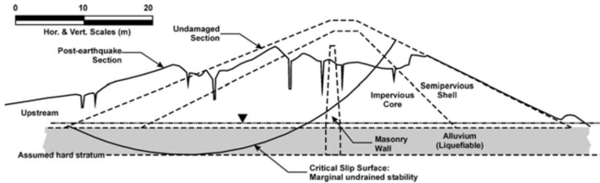
Figure 2. Cross-section of Chang Dam showing undamaged and damaged Embankment. The critical slip surface was calculated based on a post-earthquake stability analysis performed by the original author (from Singh et al., 2005).
