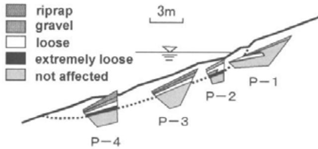
Fig.4 Cross section of the sliding failure by pit excavation investigation
