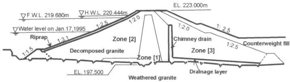
Fig.1 Cross section of the Kitayama Dam
