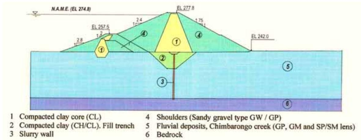
Figure 3. Embankment cross section (from Campana et al., 2011)
