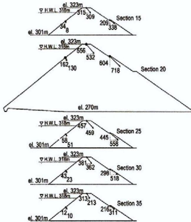
Figure 8. Movements in millimeters at five sections (from Matsumoto et al., 2011).
