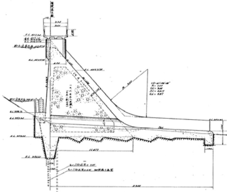
Figure 13. Cross-section of Uh Dam (from Takasu et al., 2000).
