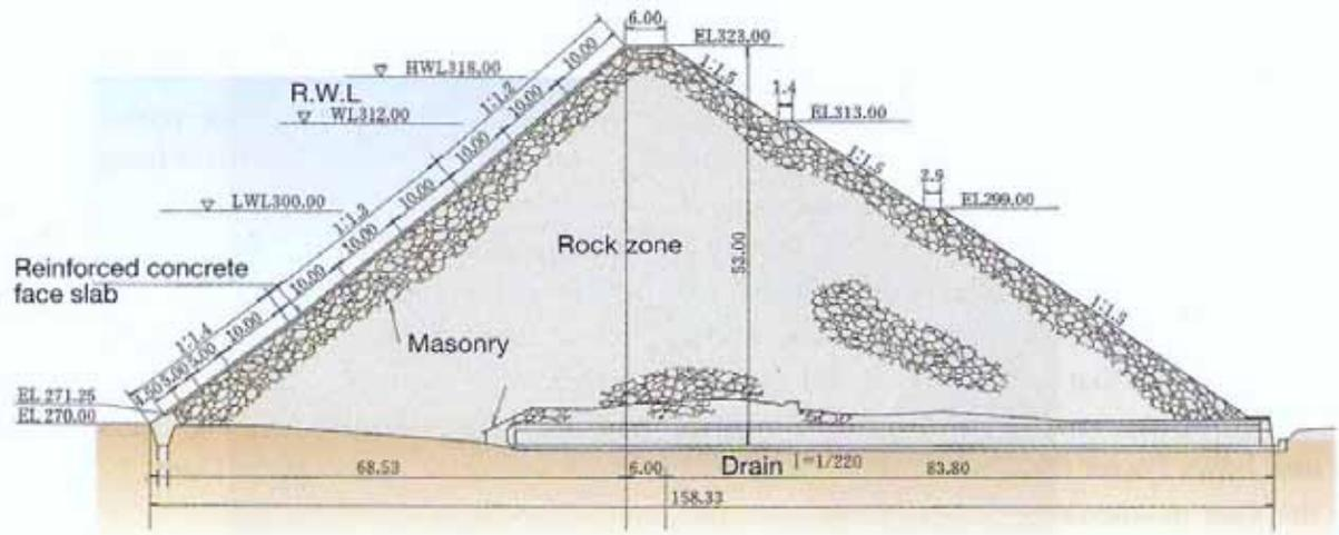
Figure 3. Embankment – maximum section (from JCOLD 2009).
