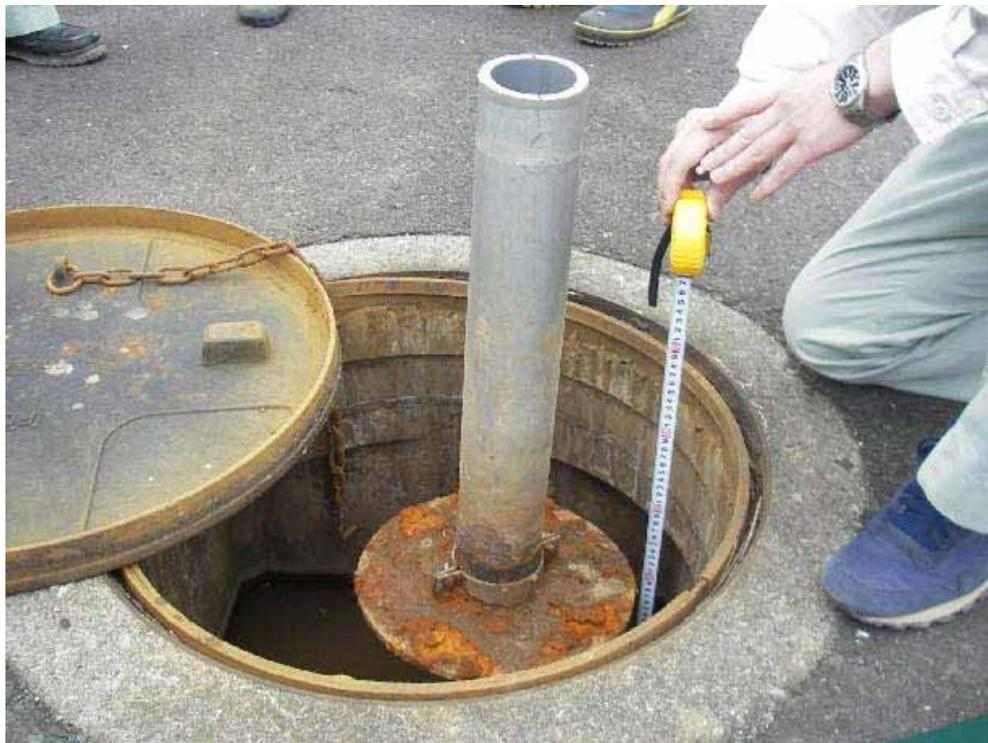
Figure 6. Settlement device (from Yamaguchi et al., 2008)
