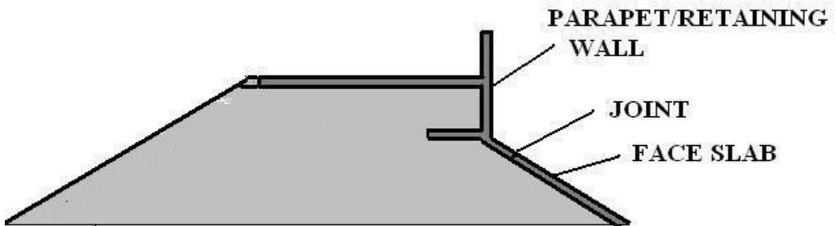
Figure 6. Schematic of pre earthquake crest detail (Babbitt).
