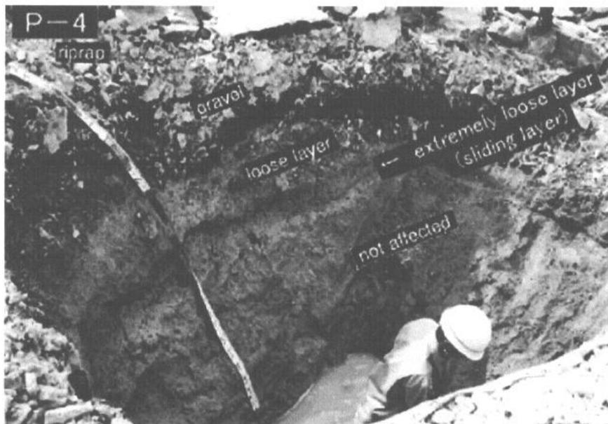
Fig.3 View of pit (P-4) excavated at the failure zone of the dam
