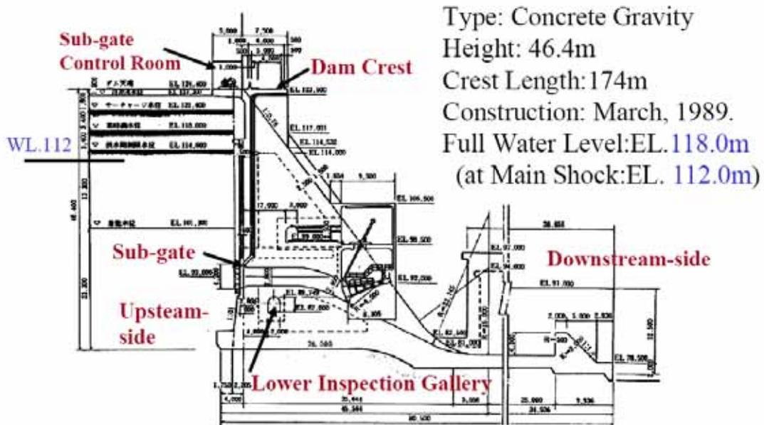
Figure 6. Section view of Kasho Dam (from Ohmachi, 2007).
