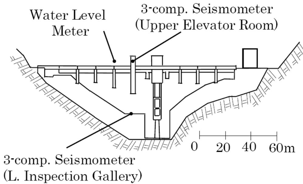
Figure 7. Profile of Kasho Dam (from Ohmachi, 2007).
