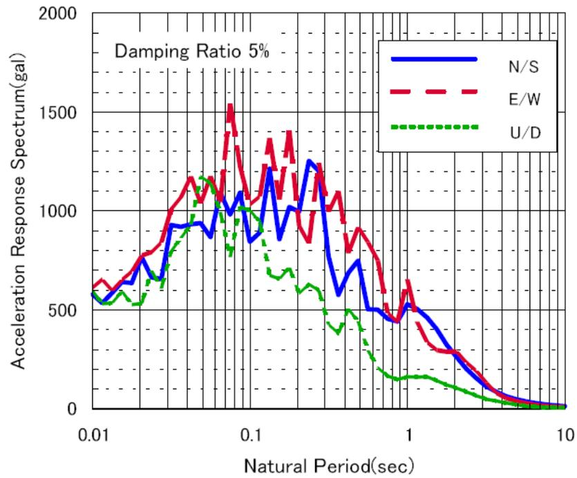
Figure 9. Acceleration response spectra at 5% damping computed from measured accelerations in the lower gallery (from Yamaguchi et al., 2002).
