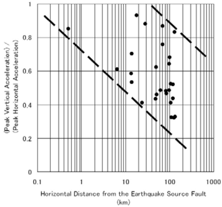
Figure 3. Ratio of vertical to horizontal peak accelerations vs. horizontal distance from the earthquake fault (from Yamaguchi et al., 2002).
