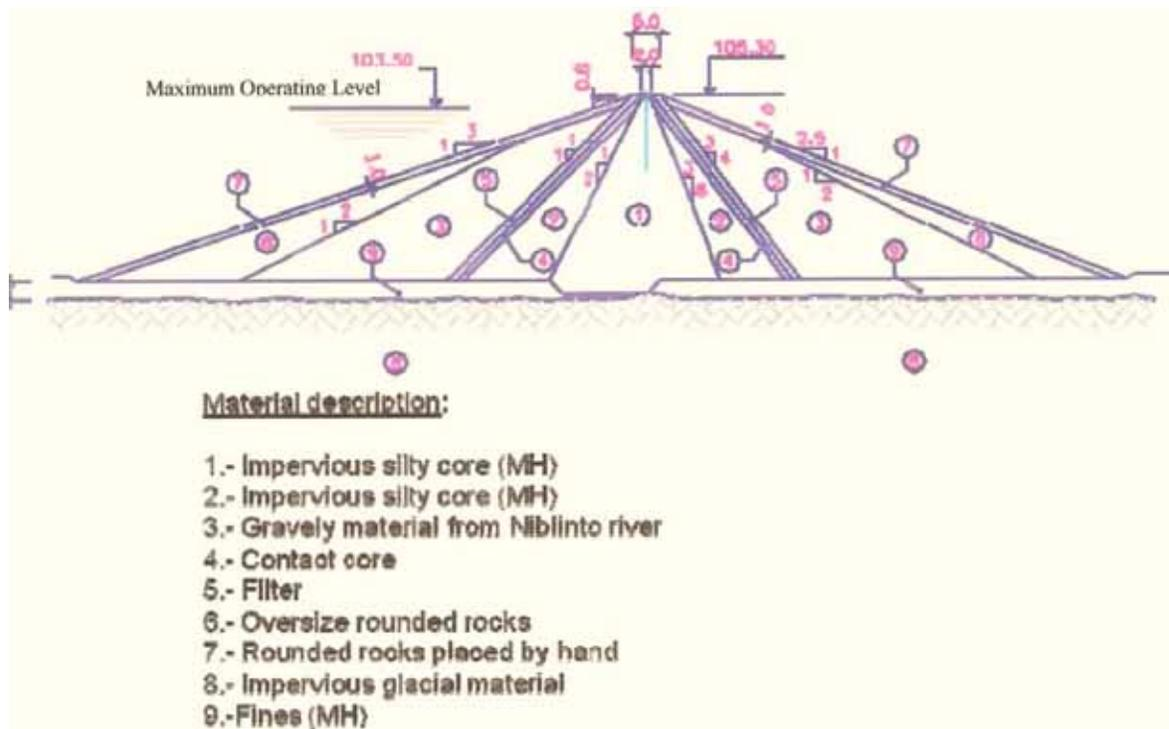
Figure 1. Embankment maximum section (from Bray et al., 2010).
