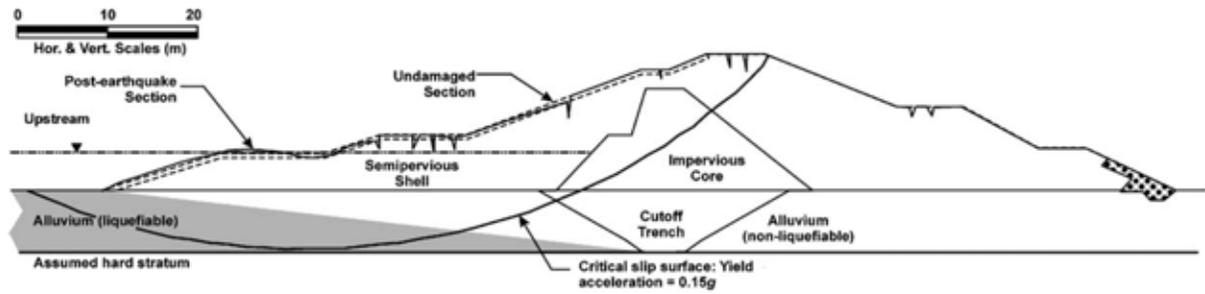
Figure 5. Cross-section of Tapar Dam showing undamaged and damaged embankment. The critical slipsurface was calculated based on a post-earthquake stability analysis performed by the original author (from Singh et al., 2005).
