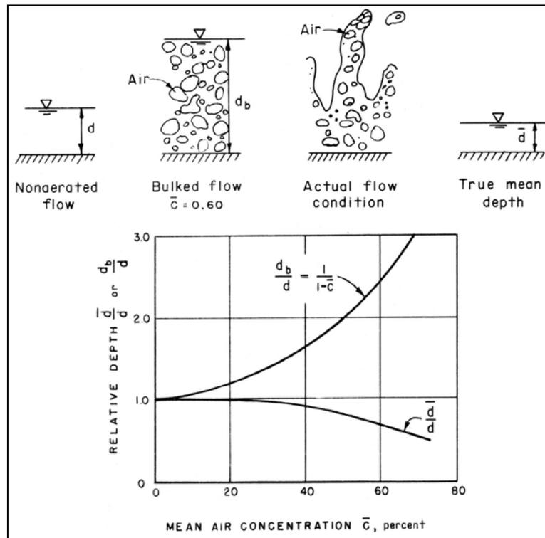
Figure F-2-4.—Air concentration in flow (Flavey 1980).
