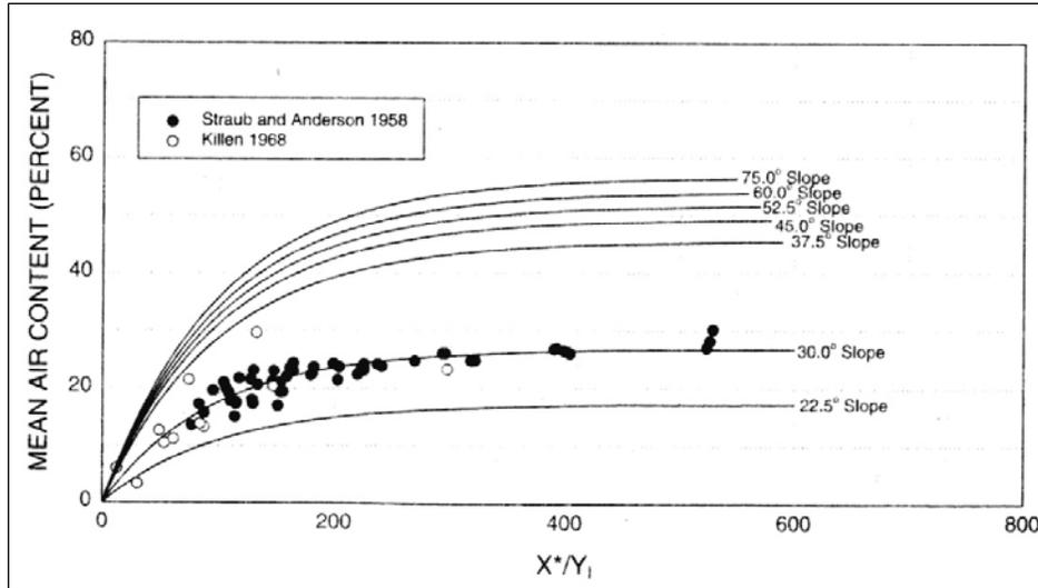
Figure F-2-2.—Mean concentration of entrained air (percent by volume) (Wilhelms and Gulliver 2005).
