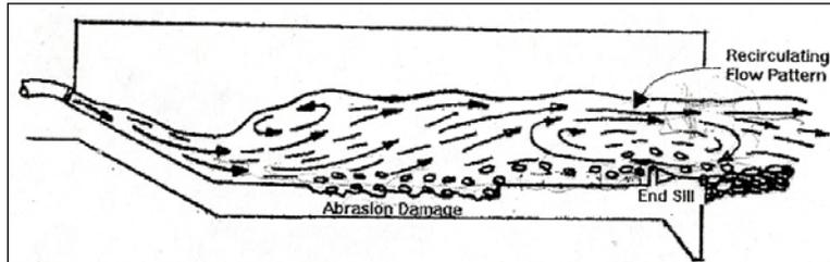
**Figure F-2-5.—Recirculating flows in hydraulic jump stilling basin.**
