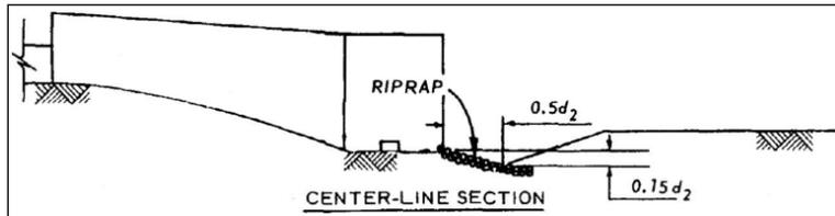
**Figure F-2-6.—Section view of stilling basin showing downstream pre-formed scour hole (plate C-43, EM 1110-2-1602, USACE 1980).**
