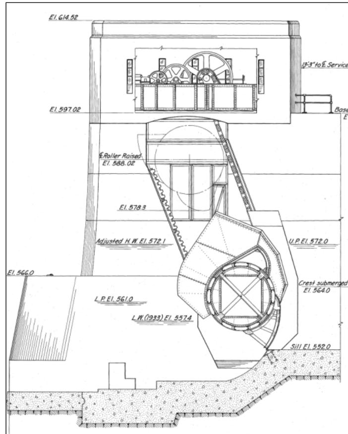
Figure G-2-4.—Cross section of a roller gate, Lock and Dam 14, Iowa (USACE 1936).
