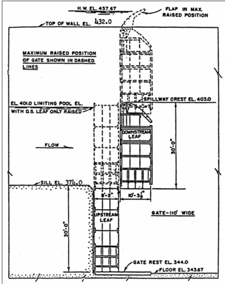
Figure G-2-6.—Submersible vertical lift gate (USACE 2006).
