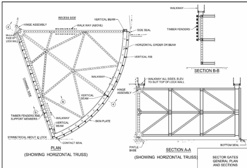
Figure G-2-11.—General plan and section of a sector gate (USACE 2014a).
