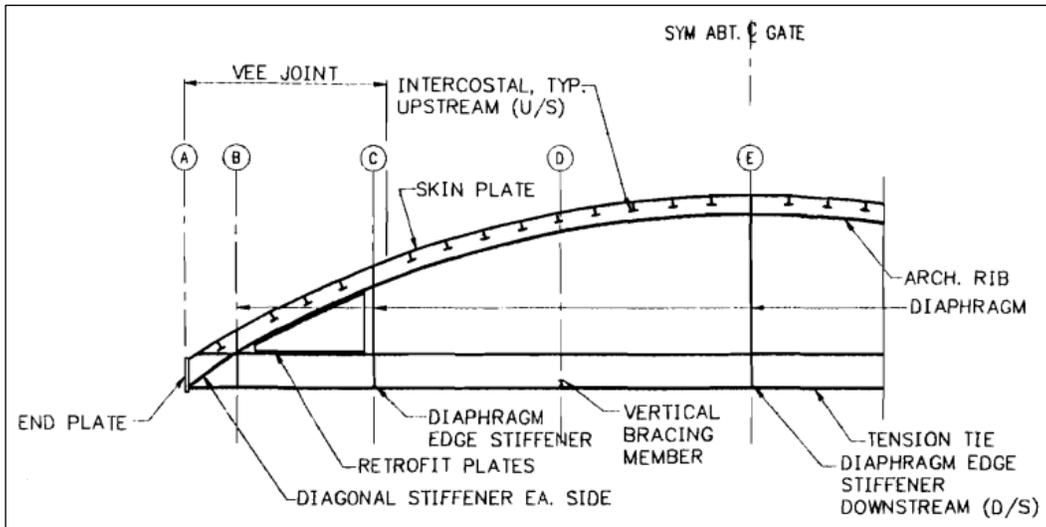
Figure G-2-16.—Vertical lift gate section at the arch frame, John Day Lock and Dam (USACE 1995).
