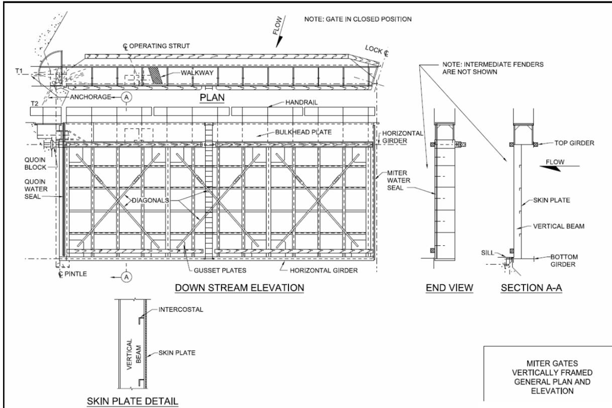
Figure G-2-9.—General plan and elevation, vertically framed miter gates (USACE 2014).
