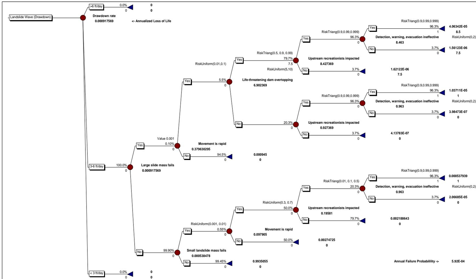
Figure H-2-1.—Example landslide event tree.
