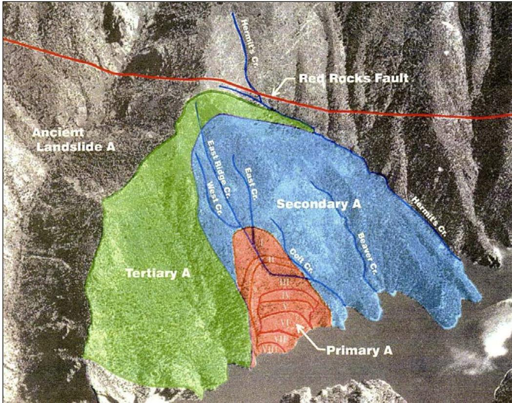
**Figure H-2-2.—Landslide masses for example (Primary A is lower portion experiencing largest movements, Secondary A is upper portion experiencing slower movements, and Tertiary A does not appear to be moving).**
