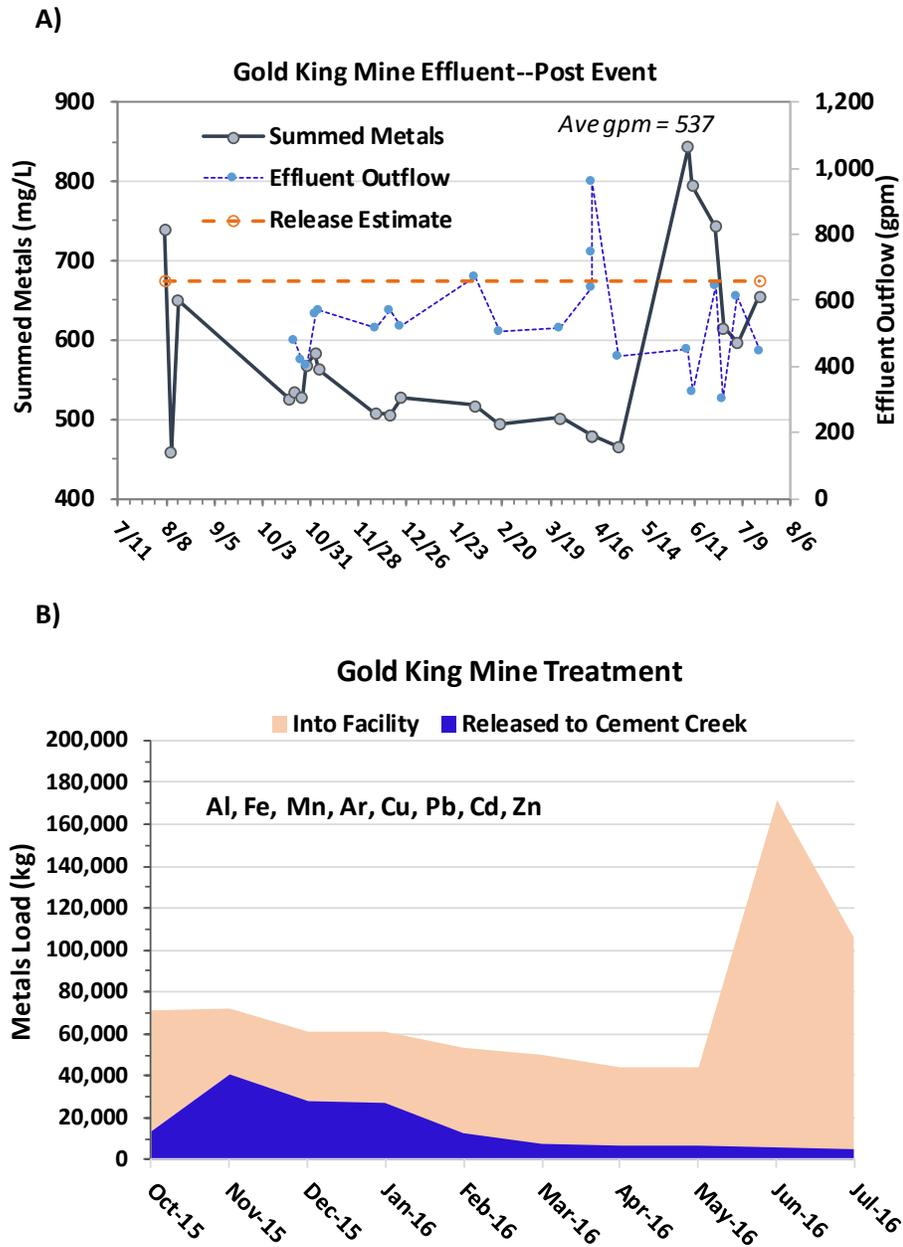
Figure 9-10. A) Weekly statistics on rate of inflow of effluent and total metals concentrations received at the Gladstone treatment facility from the Gold King Mine. B) Treatment efficiency of Gold King Mine effluent shown as inflow of metals to mass of metals released to Cement Creek.
