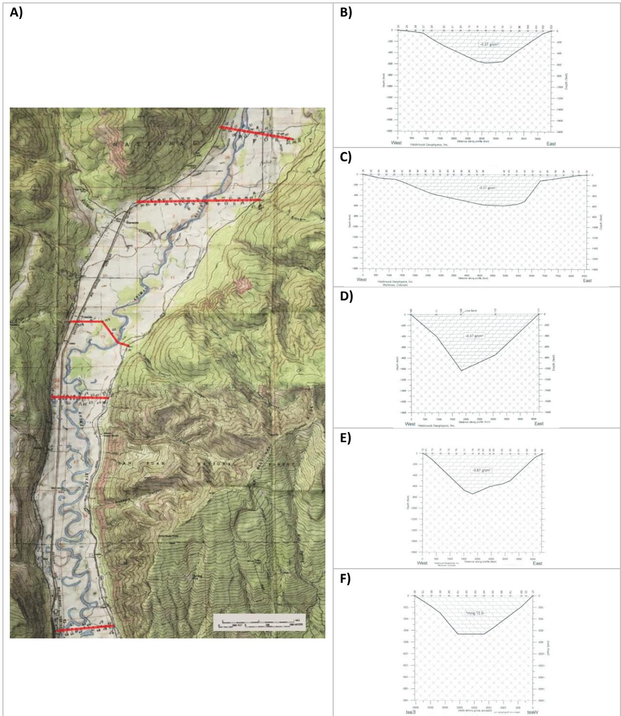
**Figure 8-3. Geophysics modeling of the shallow floodplain aquifer base elevation based on a gravity survey: A) map of the five gravity survey lines; B) line 1 gravity and depth profile – 2-layer model; C) line 2; D) line 5; E) line 3; and F) line 4. Data source: Hasbrouck Geophysics (2003).**
