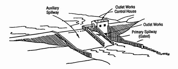
The construction materials and configuration of spillways and outlet works may differ considerably from one dam to the next.
