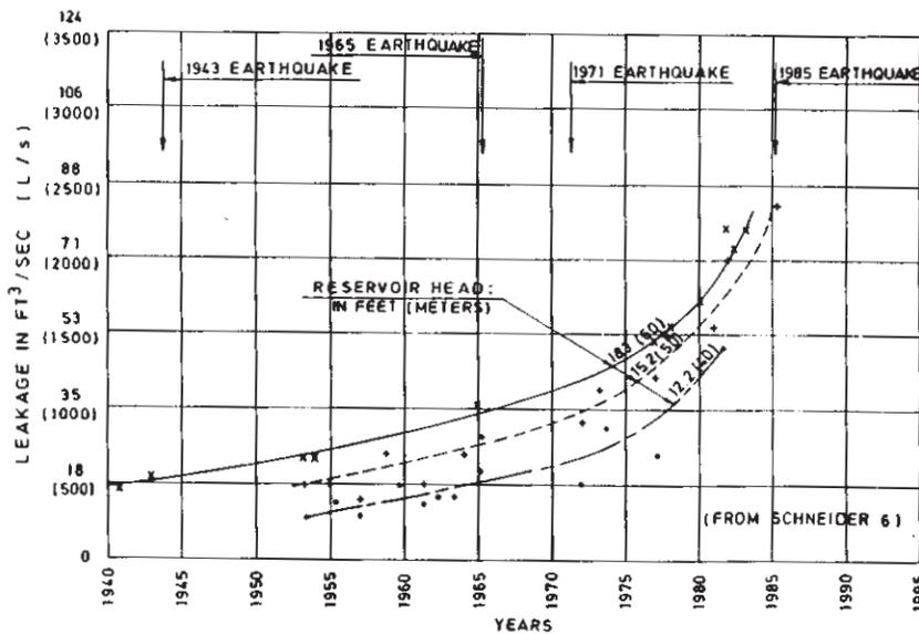
FIGURE 7 - LEAKAGE AT COGOTI DAM
