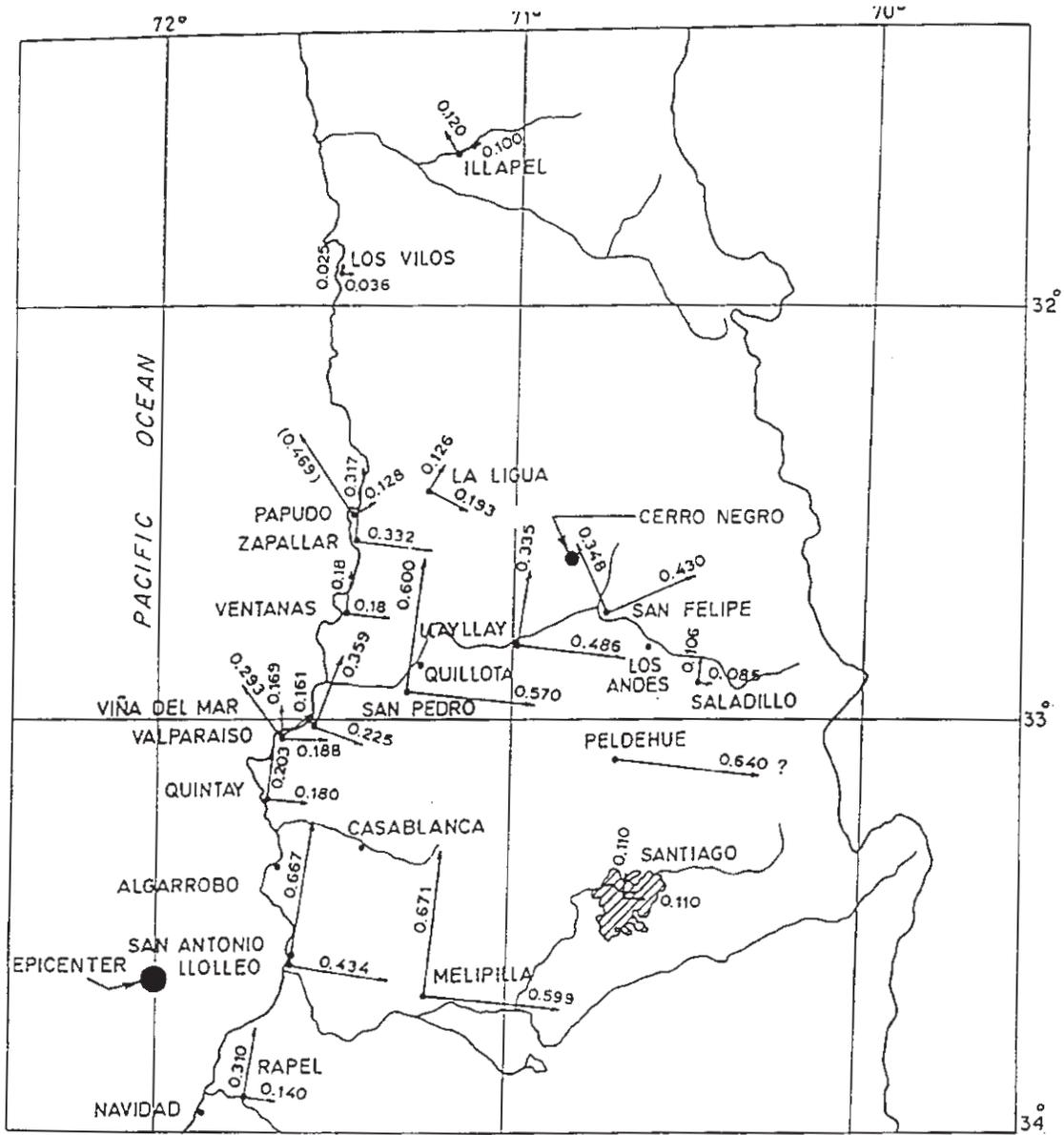
NOTES: ARROWS INDICATE DIRECTION OF RECORDED PEAK HORIZONTAL ACCELERATION, NOTED AS A FRACTION OF GRAVITY
