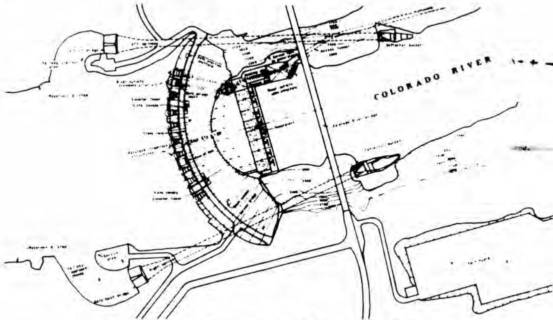
Figure 2a Plan view of Glen Canyon Dam.
