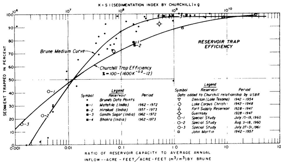
Figure 9. - Trap efficiency curves.
