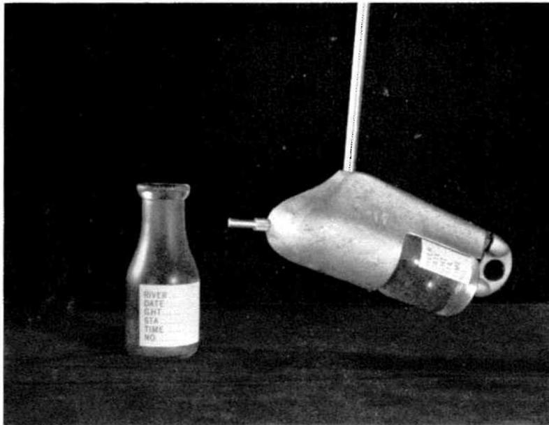
Figure 5. - Suspended sediment sampler DH-48.
