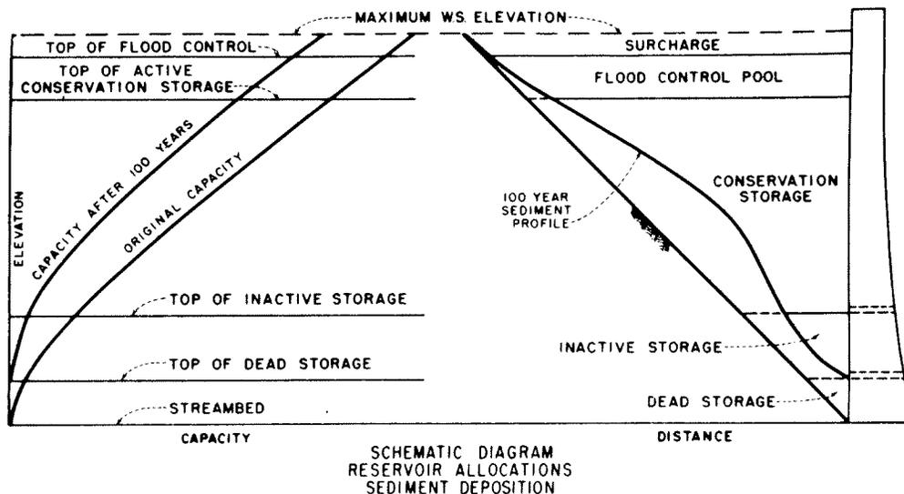
Figure 8. - Schematic diagram, reservoir allocations, sediment deposition.
