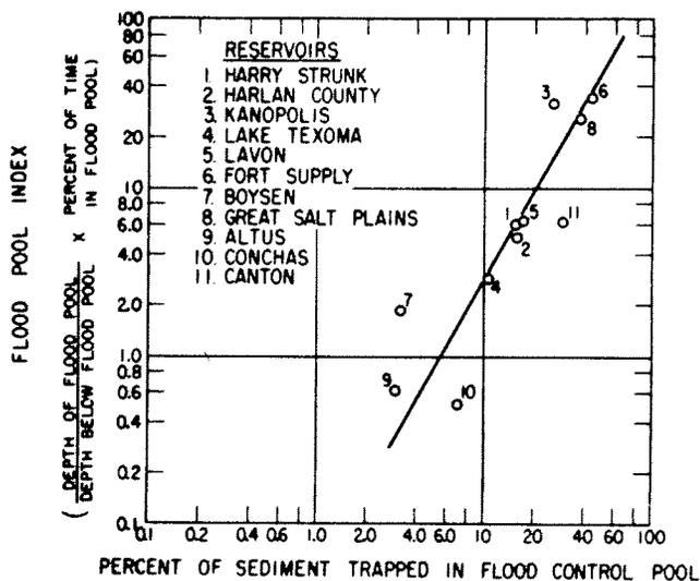
Figure 11. - Sediment deposited in flood control pool.
