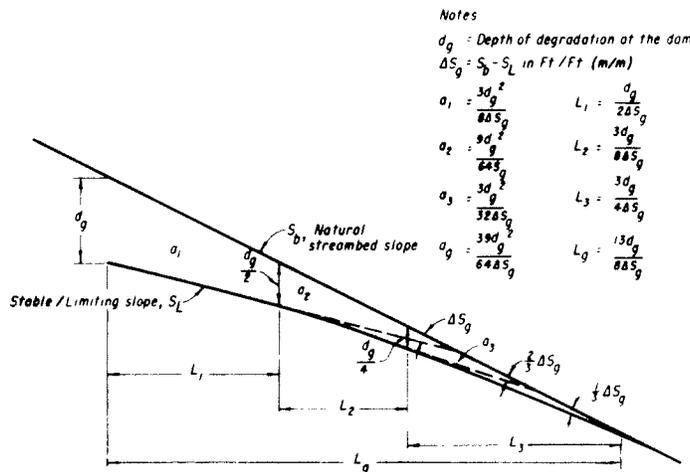
Figure 21. - Degraded channel by the three-slope method.
