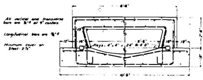
CROSS-SECTION OF SPILLWAY CULVERT
