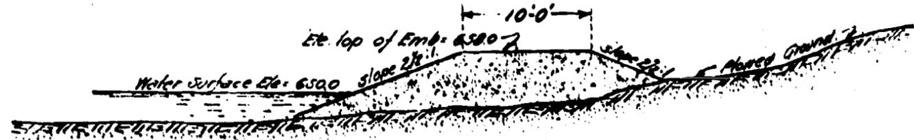
TYPICAL SECTION OF EARTH FILLED EMBANKMENT.
