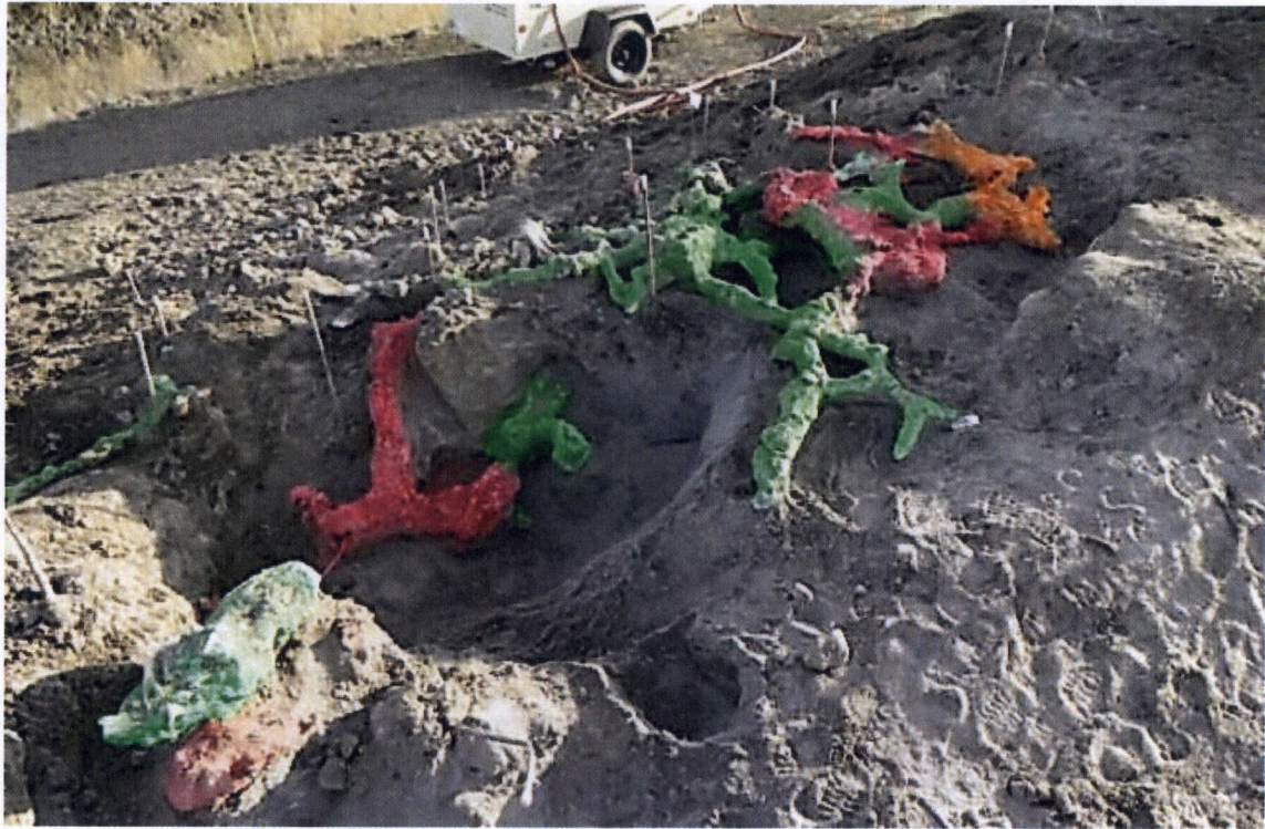
Photograph 9 – Grouted ground squirrel burrows exposed in landslide levee slope at Robbins, California
