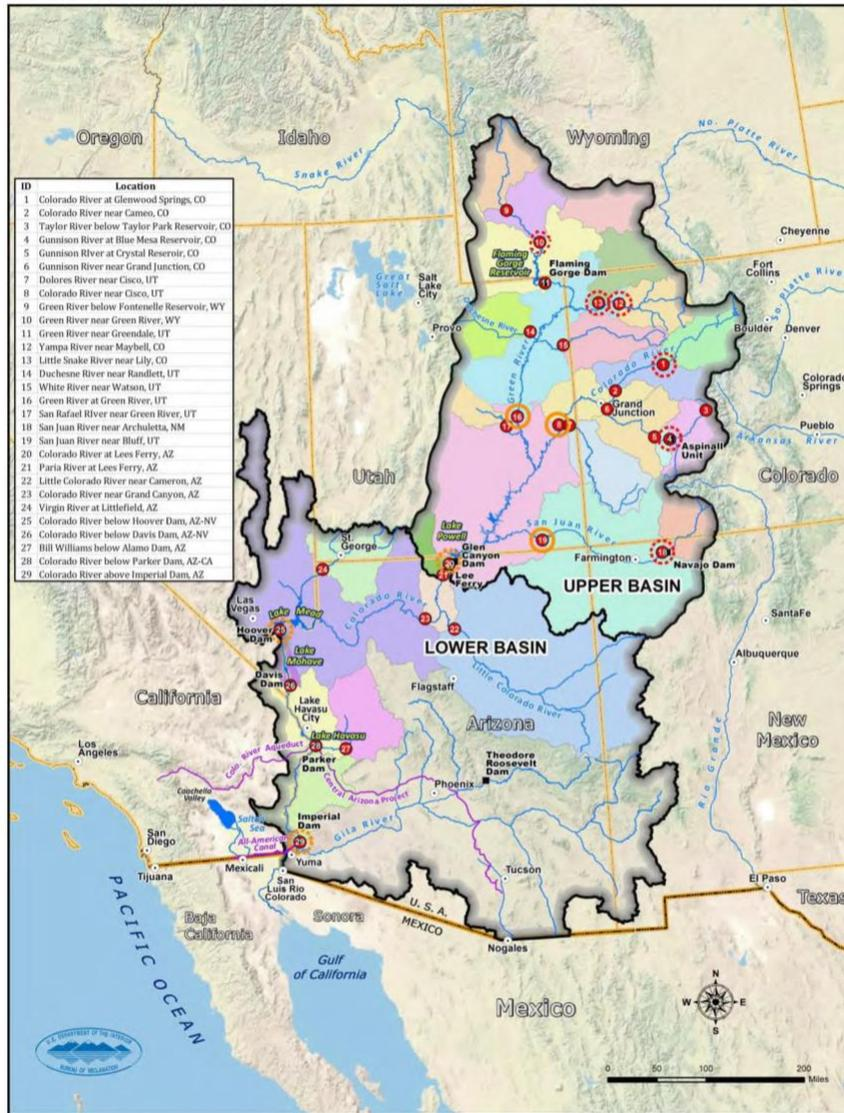
Figure 5. Map showing the Colorado River Basin in the United States and the 29 inflow nodes used in the CRSS model and showing the local-watersheds of each node. Note that the local-watershed of each node only includes the area downstream from any node further upstream.
