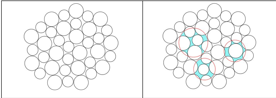
**Figure 1.** Comparison of void space for a uniformly graded soil and a broadly graded soil.
