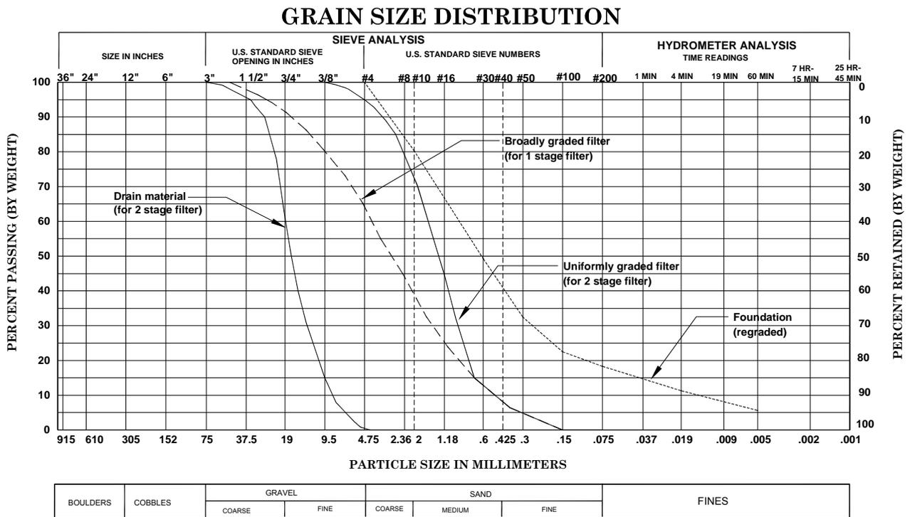
**Figure 8.** Soil gradations used in FEM analysis.
