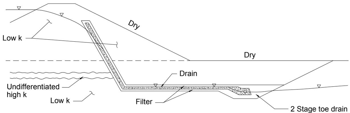
**Figure 12.** Example - Two stage chimney filter used to minimize the effect of filter barriers
