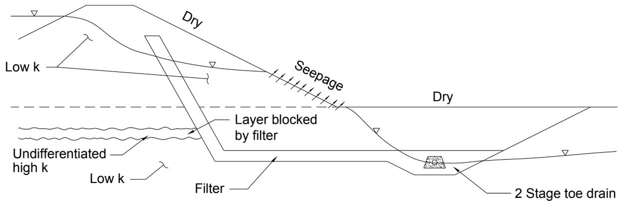
**Figure 11.** Example - Chimney filter as a filter barrier
