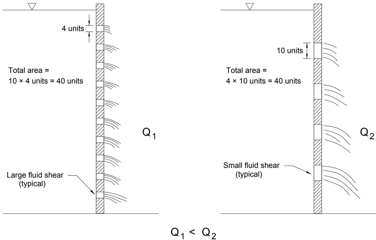
**Figure A.** Example of flow from two perforated tanks
