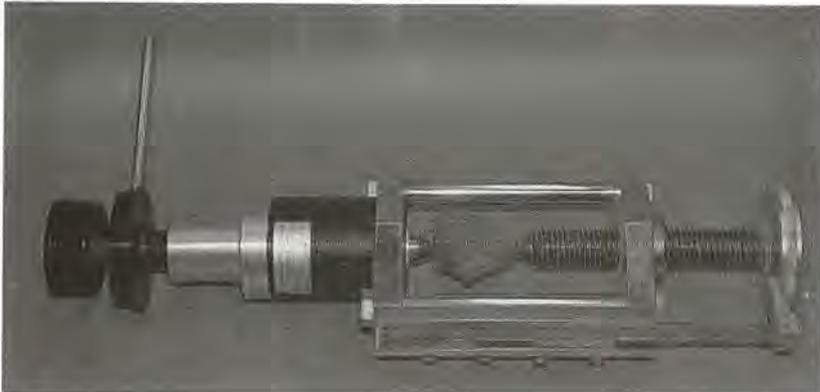
To reduce scatter in the results, the samples should respect certain length-to-diameter ( $l/d$ ) ratios:  $l/d \geq 1.4$  for cores and  $l/d$  between 1.0 and 1.4 for rock lumps when measured perpendicular to the loaded axis. In addition, when samples indicate to the geologist the potential for significant anisotropic mechanical behavior, samples should be divided and tested in groups to measure the strengths in each direction.
