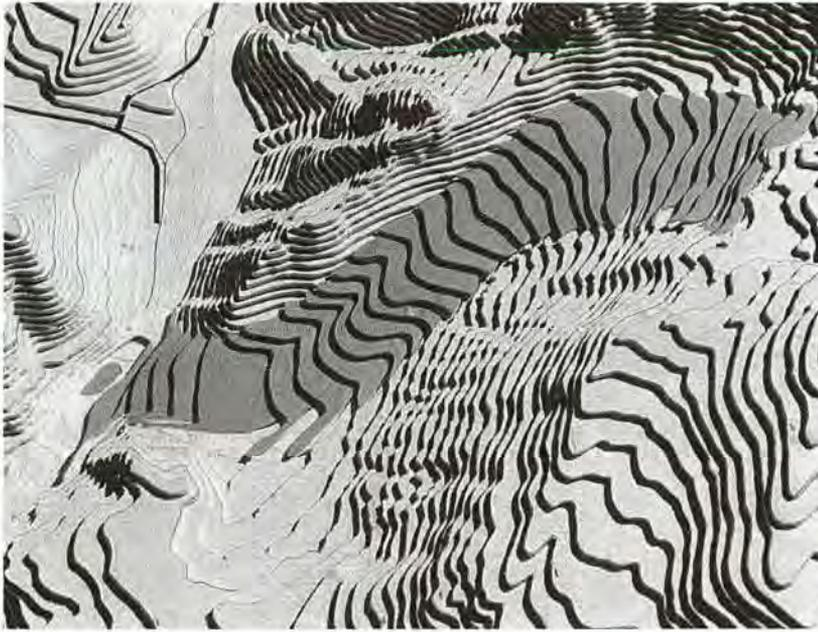
FIGURE 9-46 Example of styrofoam (foam-core) model of Thistle landslide in central Utah made by printing copies of topographic map at scale of 1:2,400 and fixing them onto sheet of styrofoam with spray adhesive. Thickness of each sheet of styrofoam was equal to vertical rise of 40 ft (12 m), and model was made with no vertical exaggeration. Equivalent sun illumination is early to mid-afternoon.
