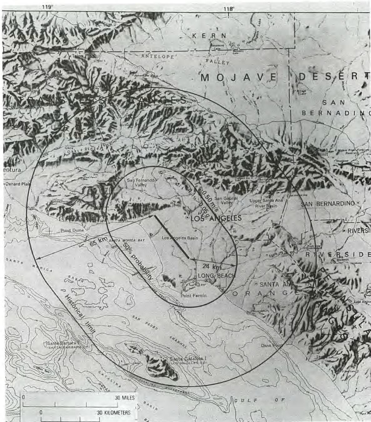
FIGURE 4-14 Map of Los Angeles basin showing predicted limit for coherent landslides from hypothetical **M** 6.5 earthquake with epicenter on northern Newport-Inglewood fault zone (solid straight line) (modified from Wilson and Keefer 1985).
