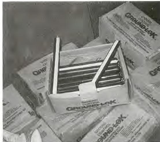
FIGURE 18-7 Resin cartridges for anchoring rock bolts.
