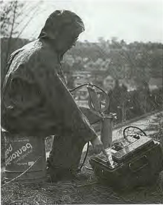
FIGURE 11-11 Digitilt inclinometer used with recorder, processor, and printer (RPP) unit (Green and Mikkelsen 1988).
