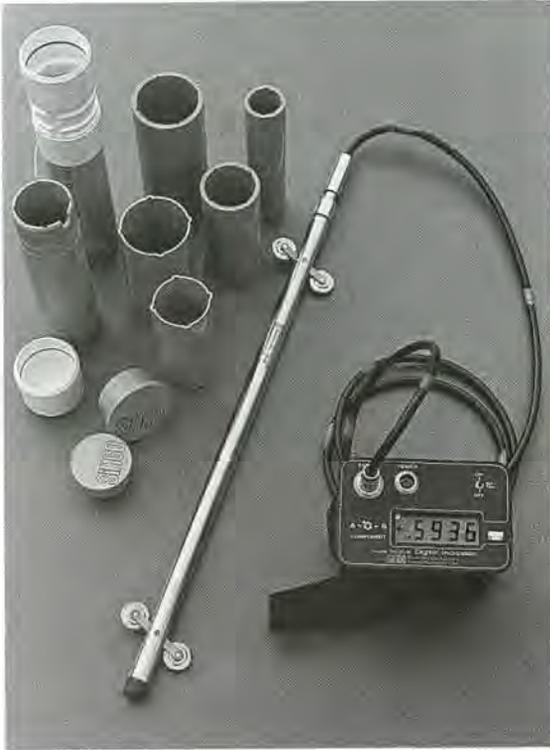
one borehole. The maximum deflection range is  $\pm 30$  degrees; the precision is reported to be  $\pm 0.01$  mm in 1 m, but this accuracy is not usually attained because of long-term drift. A more realistic maximum accuracy is about 0.04 mm in 1 m, giving a precision of 1:25,000, or about 2.5 times the precision of a probe inclinometer. Monitor and alarm consoles and telemetry systems are available for use with in-place inclinometers.
