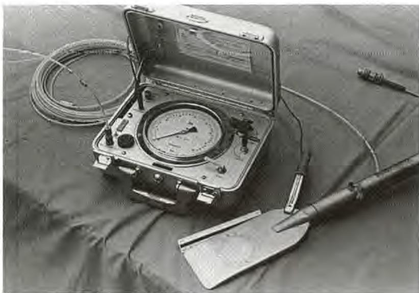
tem. The soil is then sheared by pulling the device upward through the hole. If several such tests (essentially undrained direct shear) are made on the same stratum at varying internal pressures, a Mohr failure envelope can be obtained.
