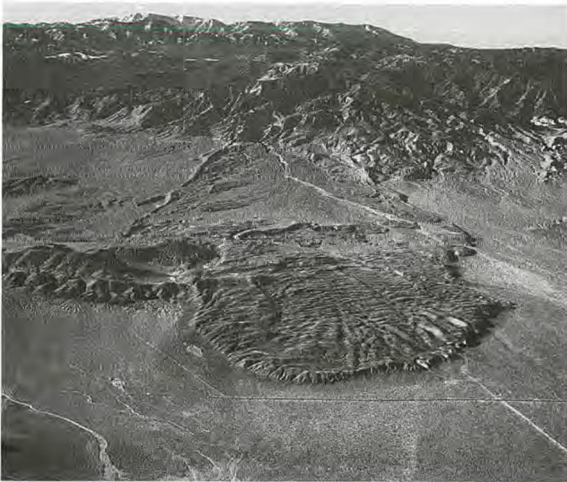
FIGURE 3-2 Blackhawk landslide: view upslope to south over lobe of dark marble breccia spread beyond mouth of Blackhawk Canyon on north slope of San Bernardino Mountains in southern California. Maximum width of lobe is 2 to 3 km; height of scarp at near edge is about 15 m [Varnes 1978, Figure 2.28 (Shelton 1966)].
