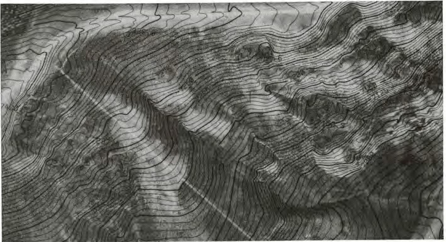
FIGURE 9-38 Example of landslide map for areal assessment, scale 1:500,000 (Harty 1991). Original map is colored and distinguishes between deep-seated, shallow, and undifferentiated landslides compiled from different sources; dots represent landslides smaller than 600 m across, and patches depict landslides larger than 600 m across. Area shown includes Ephraim Canyon, central Utah; increasing detail is shown in Figures 9-39, 9-40, 9-41, and 9-6.
