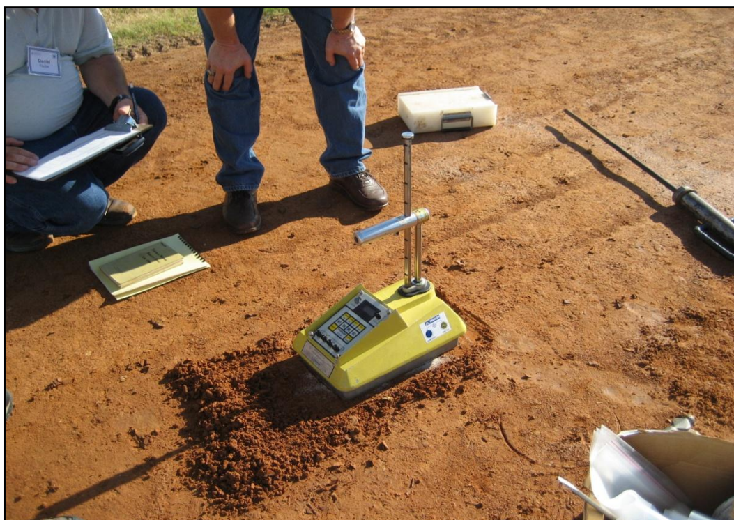
Figure 7-29. Typical nuclear moisture-density meter.
