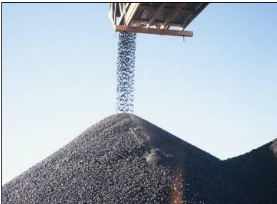
Figure 7-10. High drop height at belt discharge.
