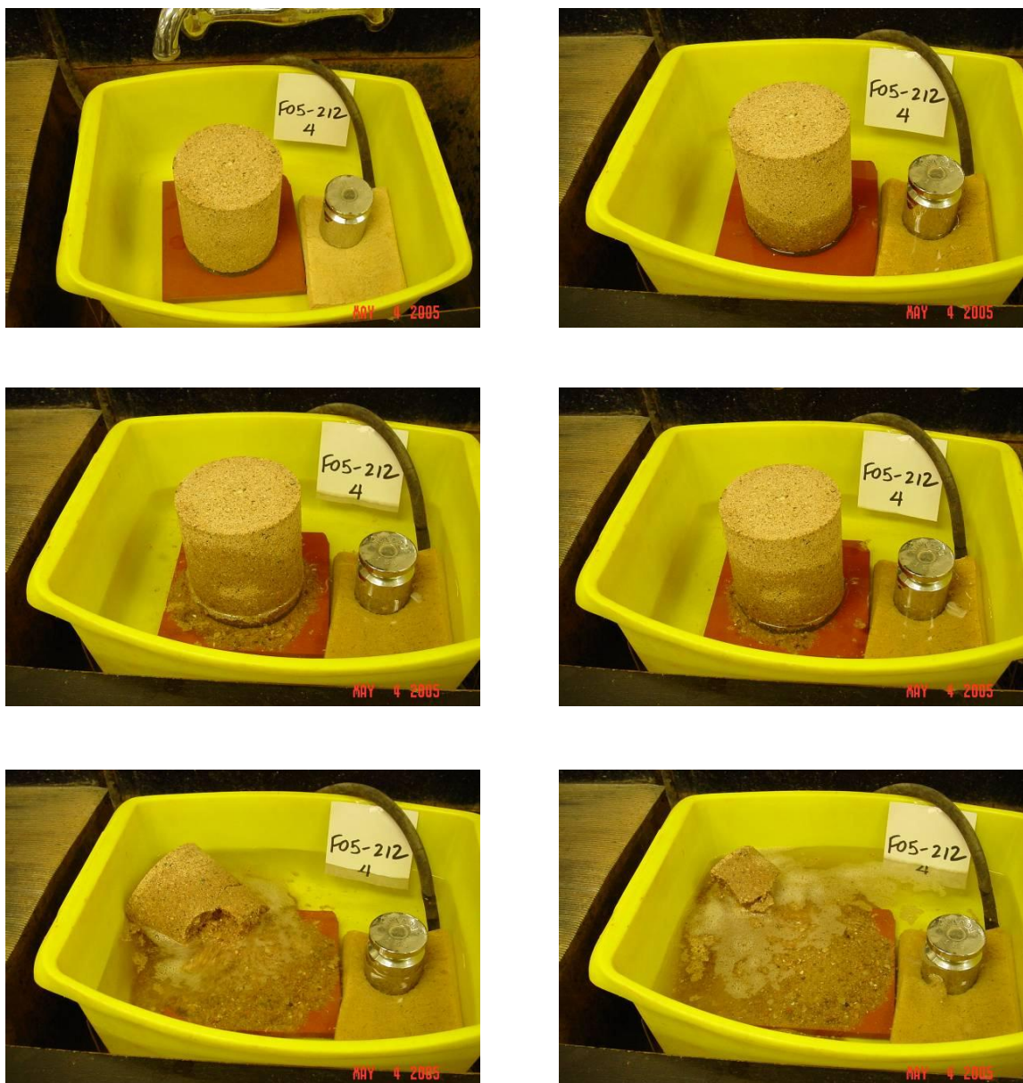
Figure 4-6. Illustration of relatively good self-healing behavior. The sample collapses relatively quickly as it is submersed.
