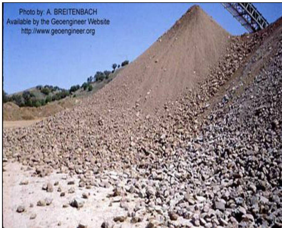
Figure 7-9. Segregation at high cone pile.
