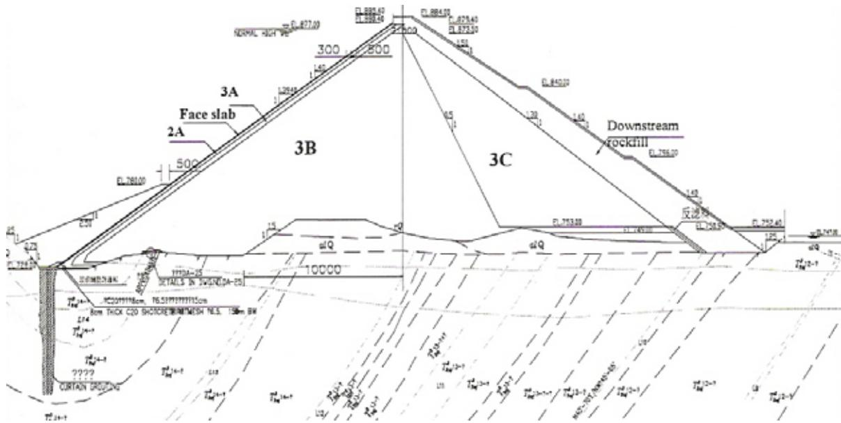
Figure 3. Embankment — maximum section (from Xu).
