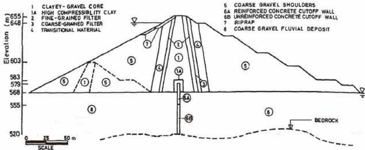
Figure 1. Typical section of embankment (from Rodriguez-Roa, 1992)
