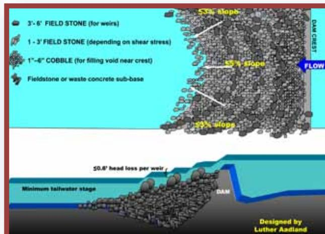
**Figure 10. Generalized conceptual design of the Rock Arch Rapids developed by Dr. Luther Aadland.**
