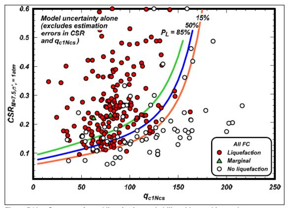
Figure B12a. Contours of equal liquefaction probability with case history data (Boulanger and Idriss, 2014). Red curve at bottom (15 percent) corresponds to cyclic resistance ratio,  $CRR_{M=7.5,\sigma'v=1atm}$ .
