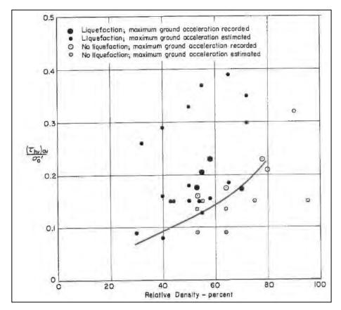
Figure 13.6.4-1. CSR and relative density of soils subjected to earthquake loading, with and without liquefaction (Seed and Peacock, 1971). Note:  $(\tau_{hv})_{av}/\sigma'_{o}$  is equivalent to 0.65  $\tau_{max}/\sigma'_{v}$ .
