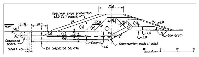
Figure G19. Geogrids for tensile reinforcement of embankment foundation, Jackson Lake Dam, Wyoming. Heavy dashed line shows location of geogrids.
