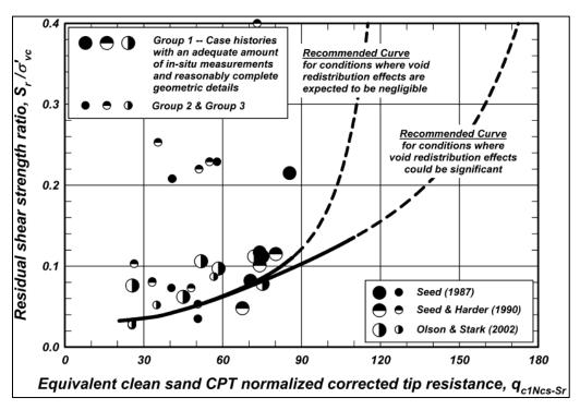
Figure F4. Idriss and Boulanger [24] correlation for  $S_{ur}/\sigma'_{vo}$  from CPT, for use with effective overburden stresses up to about 8,000 lb/ft<sup>2</sup>.
