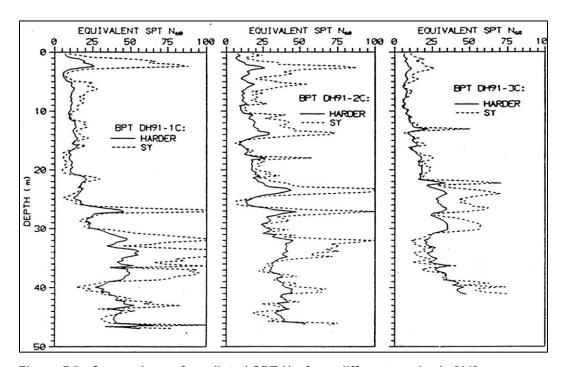
Figure D5. Comparison of predicted SPT N<sub>60</sub> from different methods [11].
