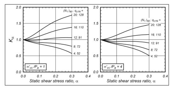
Figure 13.6.2.5-1.  $K_{\alpha}$  as a function of penetration resistance and in situ stress conditions. Note that curves for 4 atm are rotated downward from curves for 1 atm. Effective overburden stress greater than 4 atm would cause further rotation (Idriss and Boulanger, 2003, 2008).
