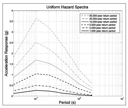
Figure A2. Example UHS. Each curve indicates the SA with a particular exceedance probability, plotted as a function of oscillation period.
