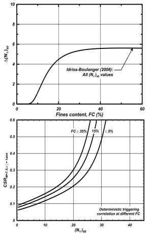
Figure C3. Adjustment of  $(N_1)_{60}$  for fines content, to yield  $(N_1)_{60cs}$  (Boulanger and Idriss, 2014).
