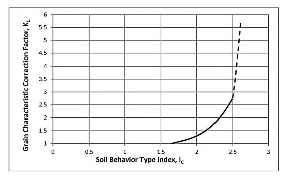
Figure B4. Grain characteristic correction factor,  $K_C$ , as a function of the Soil Behavior Type Index,  $I_C$ , based on Robertson (2009). Note that high  $K_C$  indicates high resistance to liquefaction, but not necessarily high resistance to cyclic failure of claylike soil.
