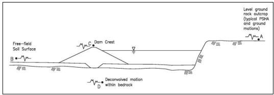
Figure 13.5.3-1. Locations requiring specific ground-motion records.
