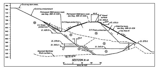
Figure G1. Stability berm and earthfill shear key with filter, Bradbury Dam, California.
