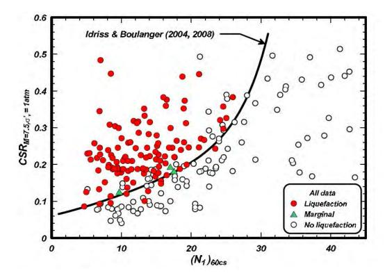
Figure C5. CRR as a function of  $(N_1)_{60cs}$ , for reference conditions of  $\sigma'_v = 1$  atm, M = 7.5, and level ground ( $\alpha = 0$ ). Curve is equivalent to the one in figure C4 for  $P_L = 15\%$  (Idriss and Boulanger, 2010).
