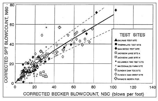
Figure D3. Correlation to estimate SPT blow count from corrected Becker blow count by Harder-Seed method [2].
