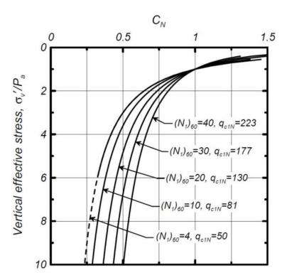
Figure C2. Overburden adjustment for SPT (Idriss and Boulanger, 2004).
