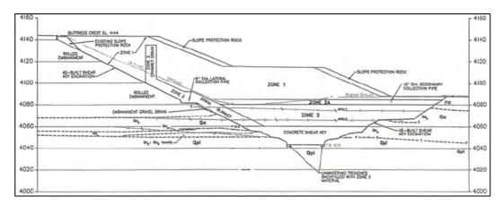
Figure G3. Partial concrete shear key, Rye Patch Dam, Nevada.
