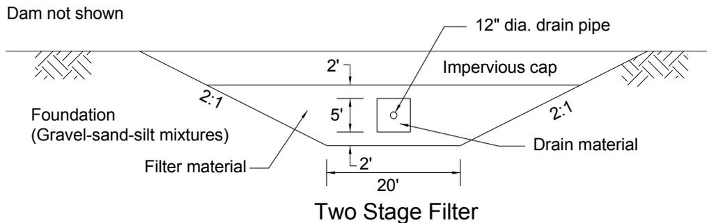
**Figure 5.** Typical two stage filter.
