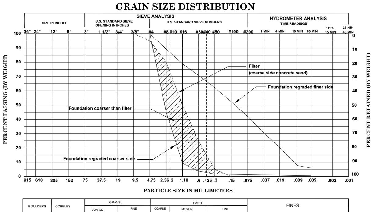
**Figure 3.** The filter barrier concept illustrated on a grain size distribution plot.
