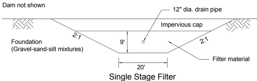
**Figure 6.** Typical single stage filter.
