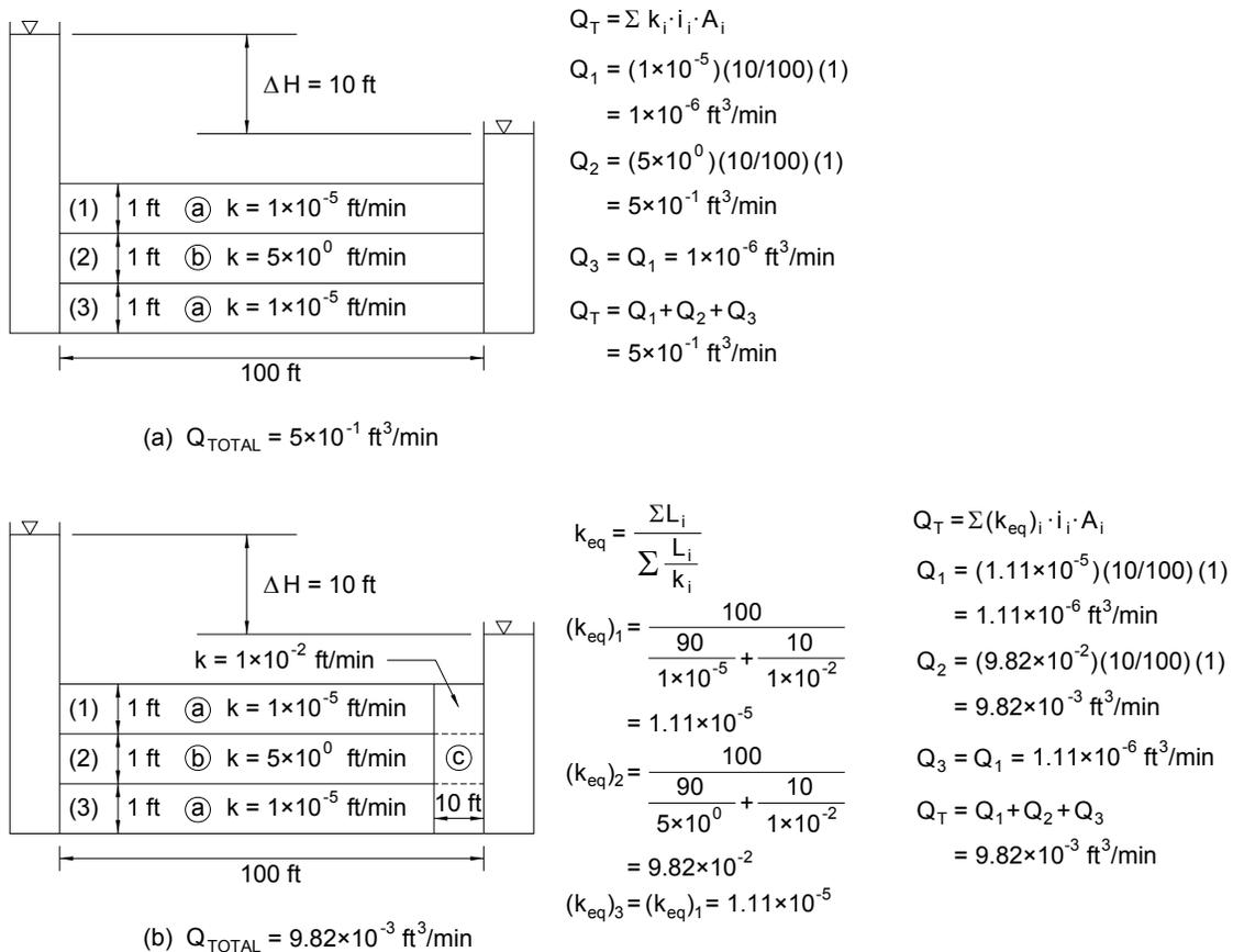
**Figure 4.** The filter barrier concept illustrated as flow through a laboratory box
