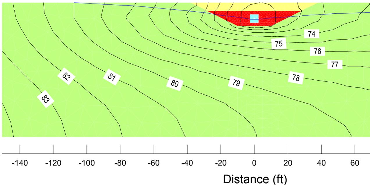
**Figure 9.** Graphical results of two stage drain FEM analysis.
