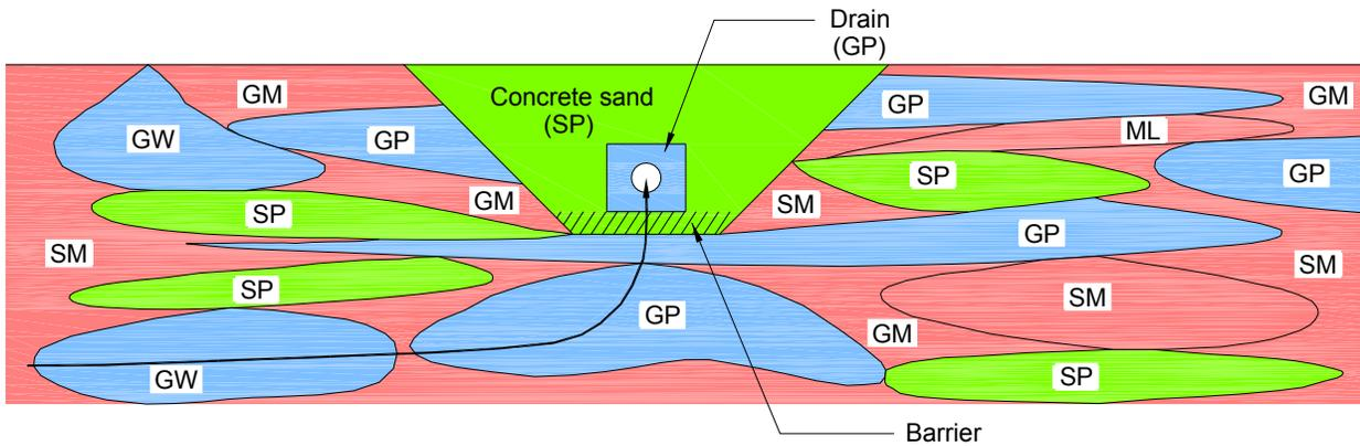
**Figure 2.** A filter for a toe drain which is acting as a barrier to a more pervious foundation layer.
