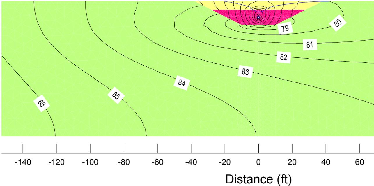
**Figure 10.** Graphical results of single stage drain FEM analysis.
