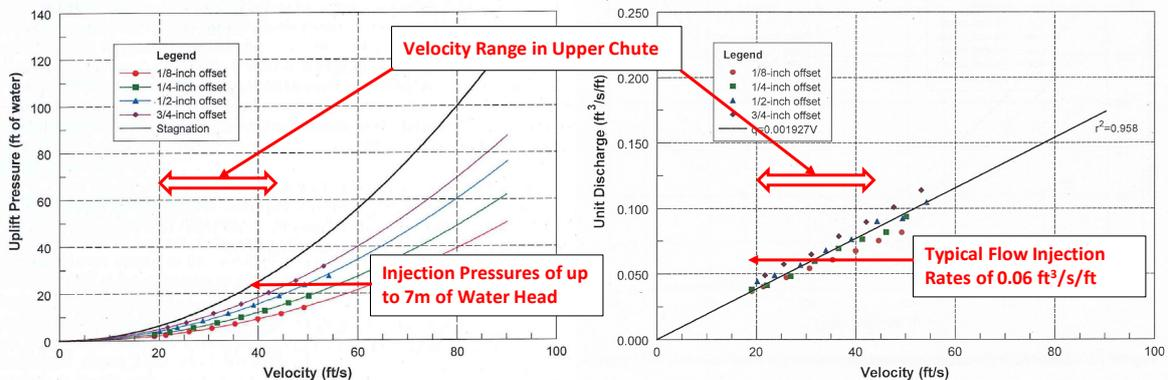
Figure 12.—Mean uplift pressure, sharp-edged geometry, vented cavity, 1/8-inch gap.
