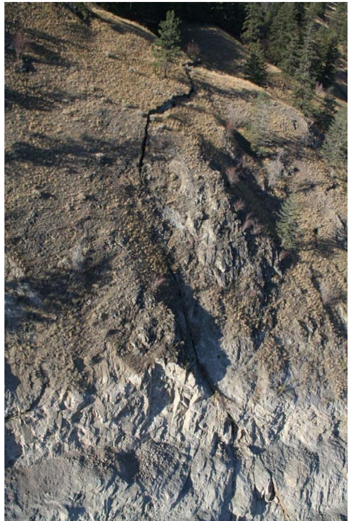
Figure 3. Tensile fracture and slip surface (Arthon Construction, Oct. 2008).
