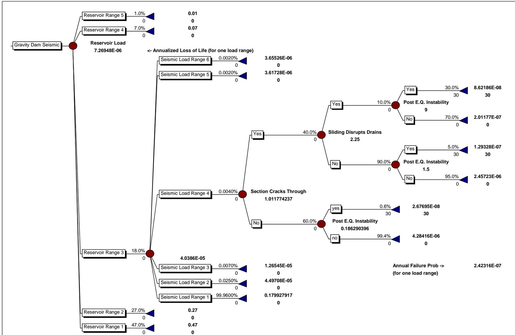
Figure E-3-3.—Concrete gravity dam instability, seismic loading.
