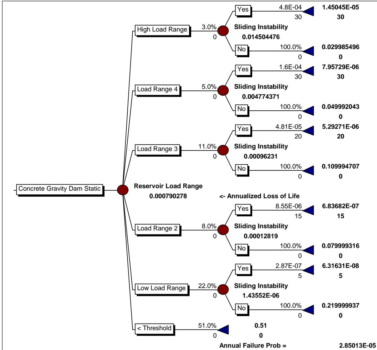
Figure E-3-1.—Concrete gravity dam instability, static load event tree.
