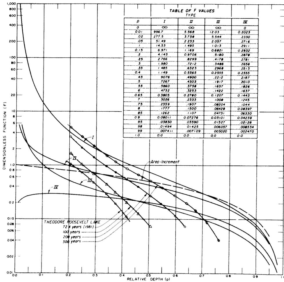
Figure 16. - Curves to determine the depth of sediment at the dam.
