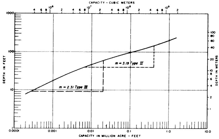
Figure 15. - Depth versus capacity for Theodore Roosevelt Lake.
