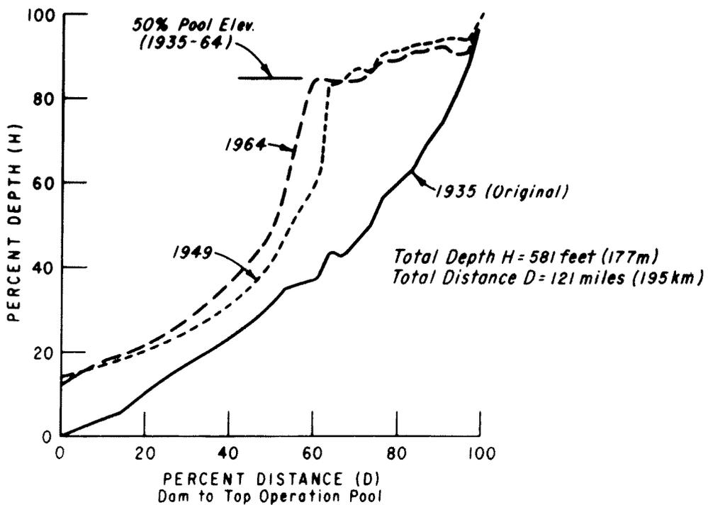
Figure 3. - Lake Mead sediment deposition profile.
