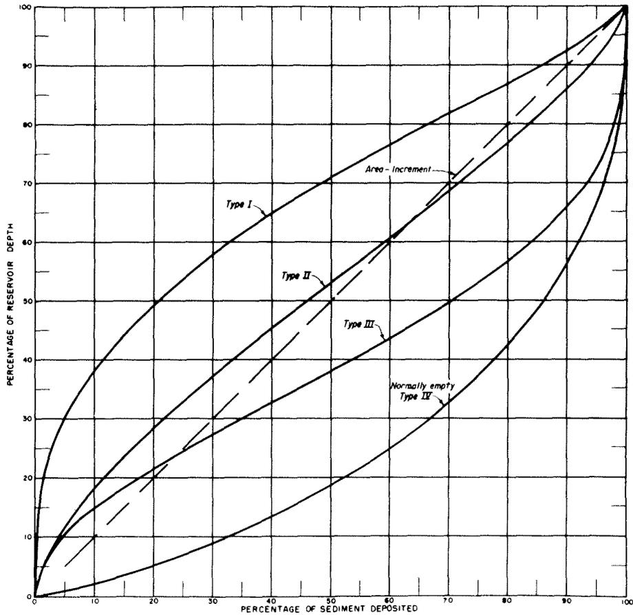
Figure 12. - Sediment distribution design curves.
