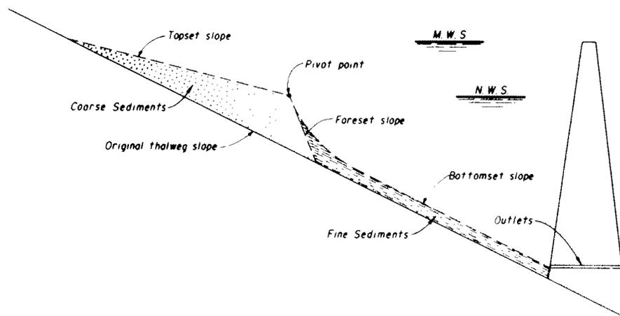
Figure 17. - Typical sediment deposition profile.
