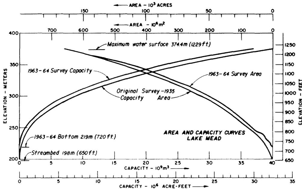
Figure 1. - Area and capacity curve for Lake Mead.
