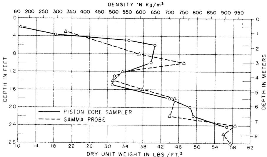
Figure 10. - Comparison of densities on Lake Mead at location 5.
