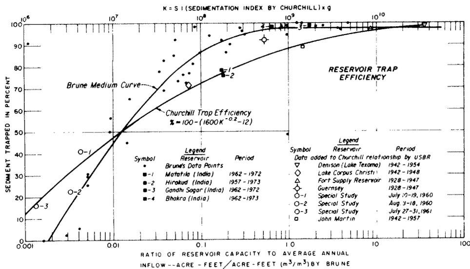
Figure 9. - Trap efficiency curves.
