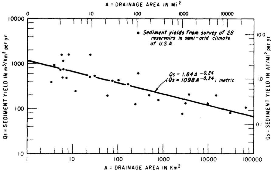
Figure 4. - Average annual sediment yield rate versus drainage area size.
