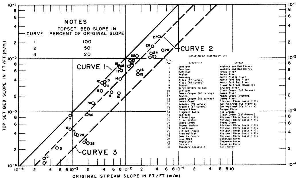
Figure 18. - Topset slope versus original stream slope from existing reservoirs.
