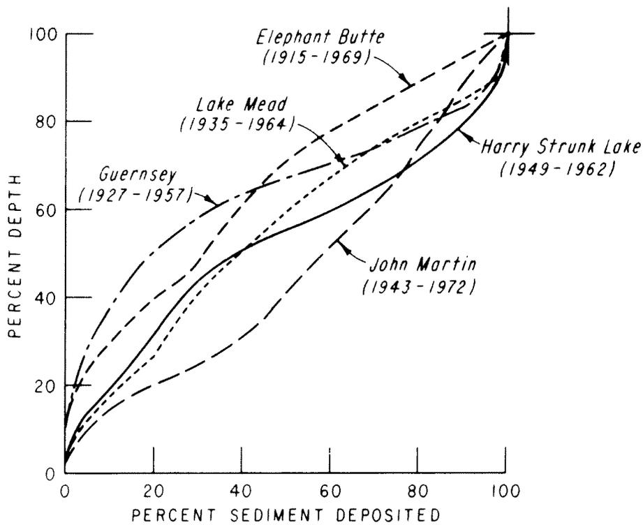
Figure 2. - Sediment distribution from reservoir surveys.
