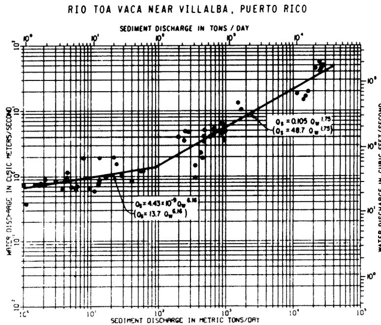
Figure 6. - Suspended sediment rating curve for Rio Toa Vaca near Villalba, Puerto Rico.
