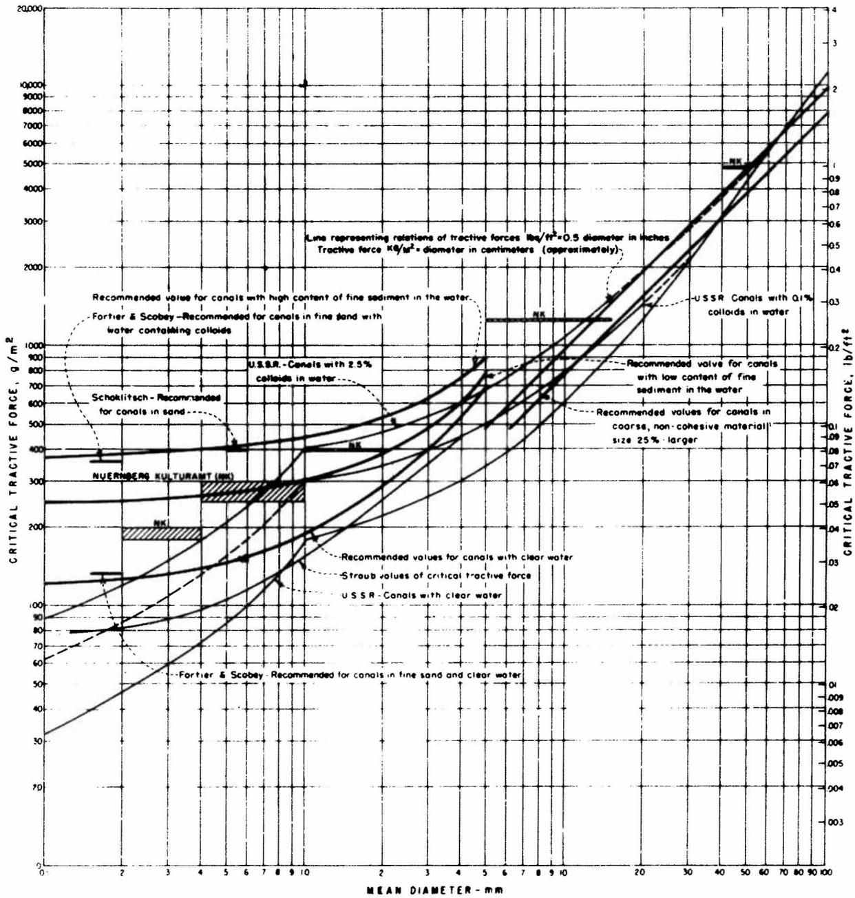
Figure 20. - Tractive force versus transportable sediment size.
