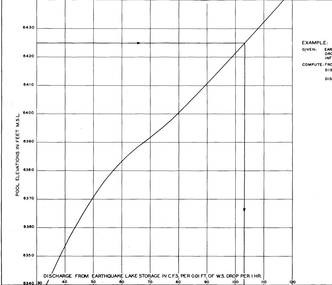
GIVEN: EARTHQUAKE LAKE POOL ELEVATION = 6425 DROP OF POOL ELEVATION = 0.20 FT. PER. HR. INFLOW FROM HEBGEN = 900 C. F. S. COMPUTE: FROM CHART:  $Q_{0.01}$  = 103.5  $\frac{C.F.S.}{0.01 \text{ FT. PER. HR.}}$ DISCHARGE FROM STORAGE:  $Q_0$  = 103.5 x 20 = 207 0 C.F.S DISCHARGE OVER CREST: Q = 2070+900 = 297 0 C.F.S.
