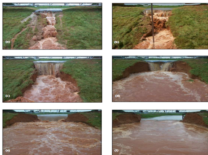
Figure 29: Stages of failure by overtopping of an embankment built of cohesive soil, as seen in a USDA field-scale test. Source: Hanson et al. (2005).
